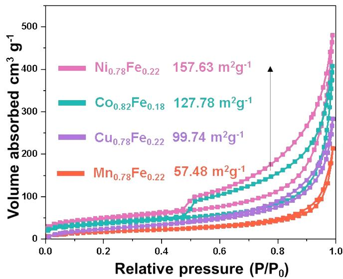
Figure S2. Nitrogen adsorption and desorption curves of  $\text{Ni}_{0.82}\text{Fe}_{0.18}$ ,  $\text{Co}_{0.82}\text{Fe}_{0.12}$ ,  $\text{Cu}_{0.78}\text{Fe}_{0.22}$  and  $\text{Mn}_{0.78}\text{Fe}_{0.22}$  samples.
