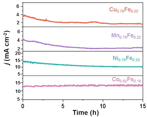
Figure S7. OER stability characterization with chronoamperometry test for 15 h.
