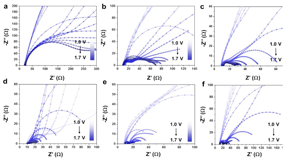
Figure S13. Nyquist plots (a-f) of  $\text{Ni}_1\text{Fe}_0$ ,  $\text{Ni}_{0.98}\text{Fe}_{0.02}$ ,  $\text{Ni}_{0.94}\text{Fe}_{0.06}$ ,  $\text{Ni}_{0.78}\text{Fe}_{0.22}$ ,  $\text{Ni}_{0.65}\text{Fe}_{0.35}$  and  $\text{Ni}_{0.56}\text{Fe}_{0.44}$  samples.
