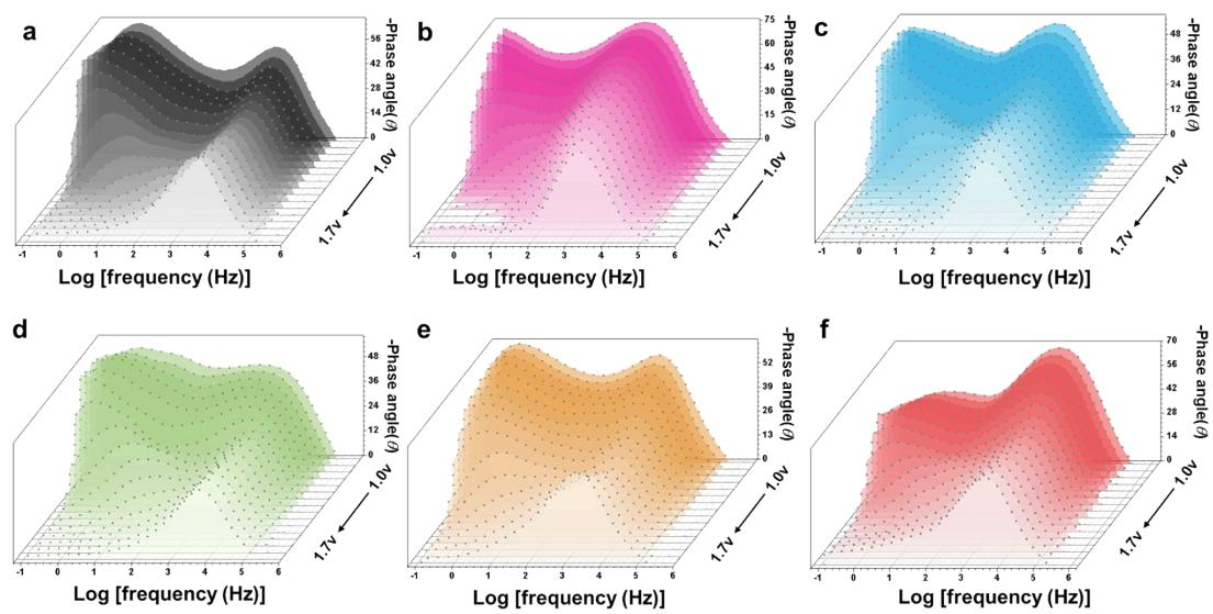
Figure S11. Bode plots of bare GC electrode, Fe, Mn,  $Mn_{0.78}Fe_{0.22}$ , Cu and  $Cu_{0.78}Fe_{0.22}$  samples.
