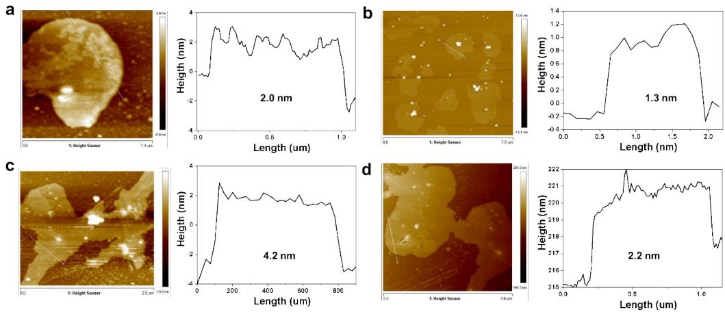
Figure S3. AFM images (a-d) of  $\text{Co}_{0.82}\text{Fe}_{0.18}$ ,  $\text{Ni}_{0.78}\text{Fe}_{0.22}$ ,  $\text{Cu}_{0.78}\text{Fe}_{0.22}$ , and  $\text{Mn}_{0.78}\text{Fe}_{0.22}$  samples.
