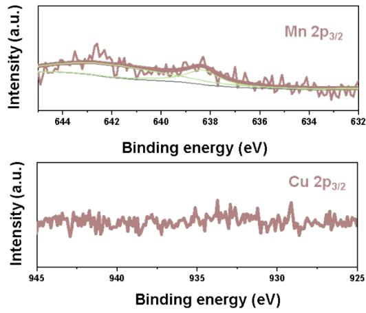
Figure S8. High-resolution XPS spectrums of Mn 2p<sub>3/2</sub> and Cu 2p<sub>3/2</sub> of Mn<sub>0.78</sub>Fe<sub>0.22</sub> and Cu<sub>0.78</sub>Fe<sub>0.22</sub> samples after OER reaction.
