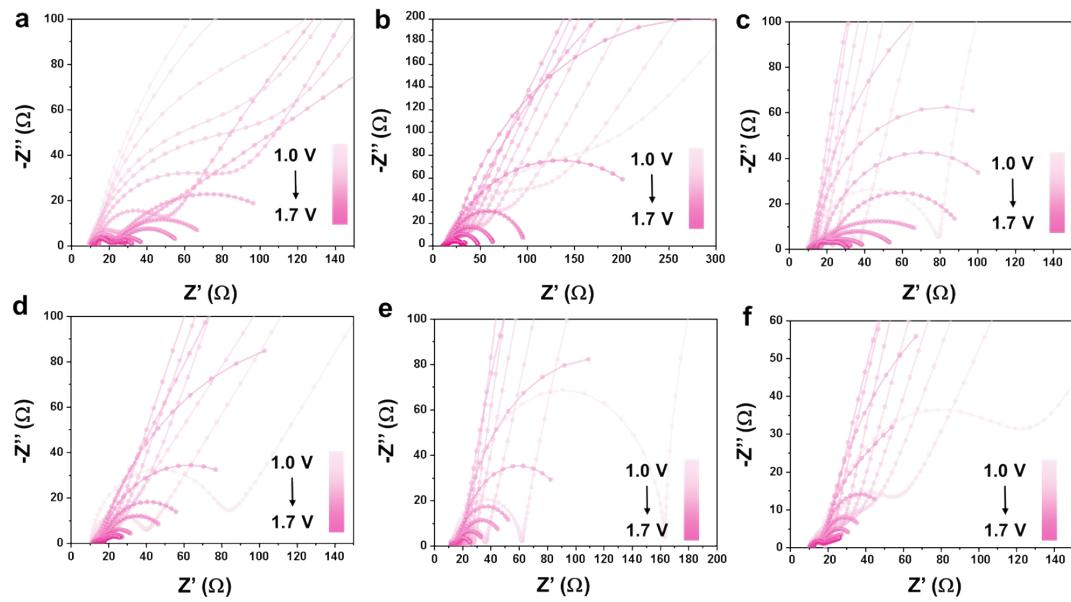
Figure S12. Nyquist plots (a-f) of  $\text{Co}_1\text{Fe}_0$ ,  $\text{Co}_{0.99}\text{Fe}_{0.01}$ ,  $\text{Co}_{0.96}\text{Fe}_{0.04}$ ,  $\text{Co}_{0.82}\text{Fe}_{0.18}$ ,  $\text{Co}_{0.71}\text{Fe}_{0.29}$  and  $\text{Co}_{0.64}\text{Fe}_{0.36}$  samples.
