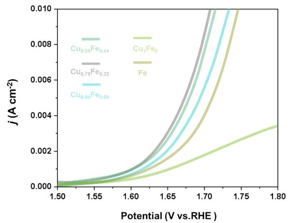
Figure S5. Polarization curves at 5  $\text{mV s}^{-1}$  for  $\text{Cu}_{1-x}\text{Fe}_x$ -LDHs.
