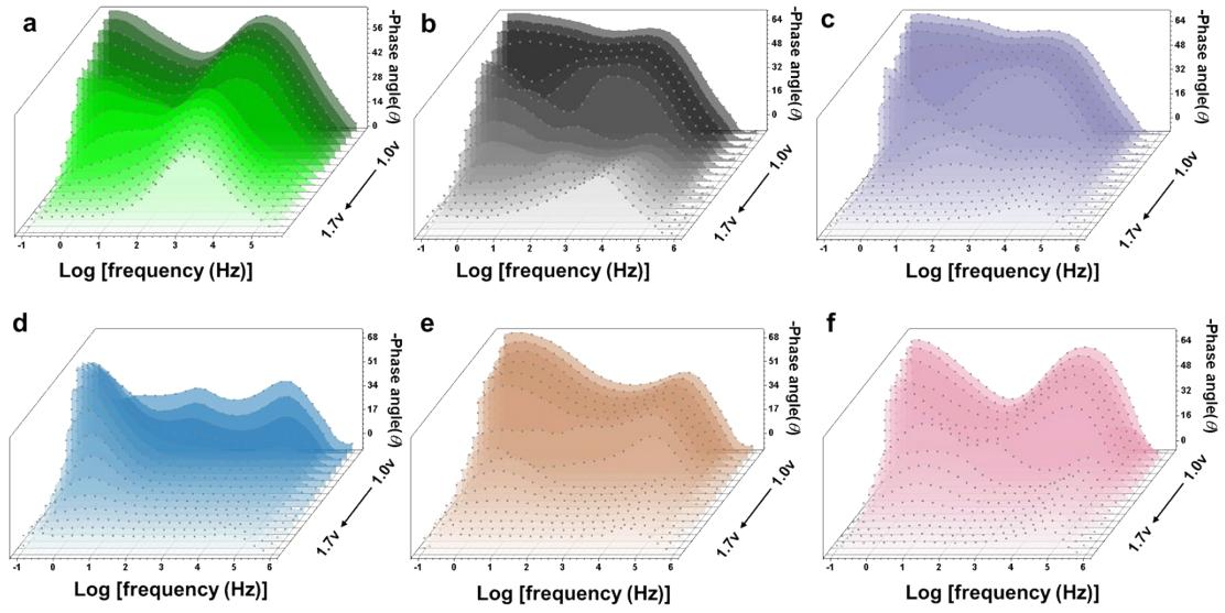
Figure S10. Bode plots of  $\text{Ni}_1\text{Fe}_0$ ,  $\text{Ni}_{0.98}\text{Fe}_{0.02}$ ,  $\text{Ni}_{0.94}\text{Fe}_{0.06}$ ,  $\text{Ni}_{0.78}\text{Fe}_{0.22}$ ,  $\text{Ni}_{0.65}\text{Fe}_{0.35}$  and  $\text{Ni}_{0.56}\text{Fe}_{0.44}$  samples.
