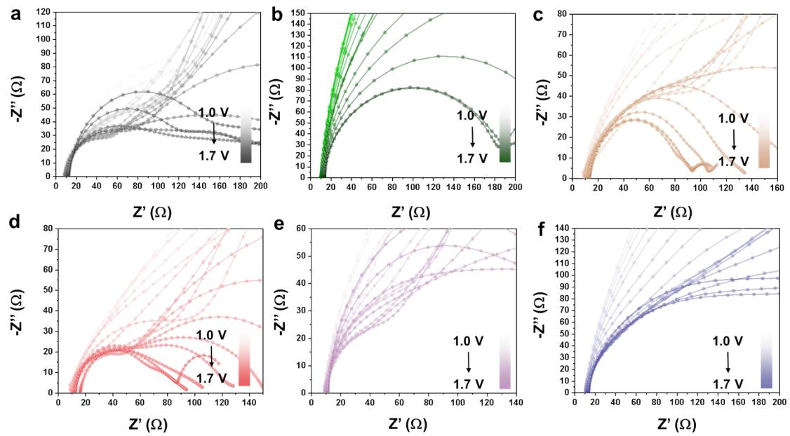
Figure S14. Nyquist plot of bare GC electrode, Fe, Mn, Mn<sub>0.78</sub>Fe<sub>0.22</sub>, Cu and Cu<sub>0.78</sub>Fe<sub>0.22</sub> samples.
