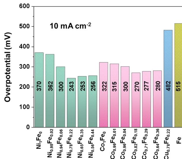
Figure S6. Overpotentials at 10 mA cm<sup>-2</sup> of different LDH samples.
