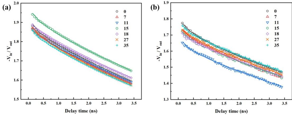
**Fig. S2** Fitting curves of  $-V_{in}/V_{out}$ -delay time for TDTR measurement of (a) as-grown and (b) annealed 2D bismuth antimonide.  $V_{in}$  and  $V_{out}$  represent in-phase and out-of-phase signals, respectively. The open symbols and the solid lines denote measured data and thermal model fitting result. Measurement conditions: modulation frequency: 1.72 MHz; pump beam spot size: 10  $\mu\text{m}$ ; probe spot size: 6.0  $\mu\text{m}$ .
