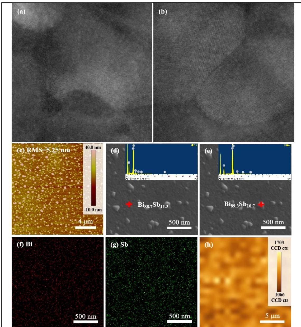
**Fig. S1 (a&b) TEM images of 2D  $\text{Bi}_{82}\text{Sb}_{18}$ . (c) AFM image of 2D  $\text{Bi}_{82}\text{Sb}_{18}$ , showing a roughness of 5.25 nm. (d&e) Point EDS results of flat area and the protruded grains in  $\text{Bi}_{89}\text{Sb}_{11}$ . (f&g) EDS mapping of 2D  $\text{Bi}_{65}\text{Sb}_{35}$ . (h) Raman mapping of 2D  $\text{Bi}_{82}\text{Sb}_{18}$ .**
