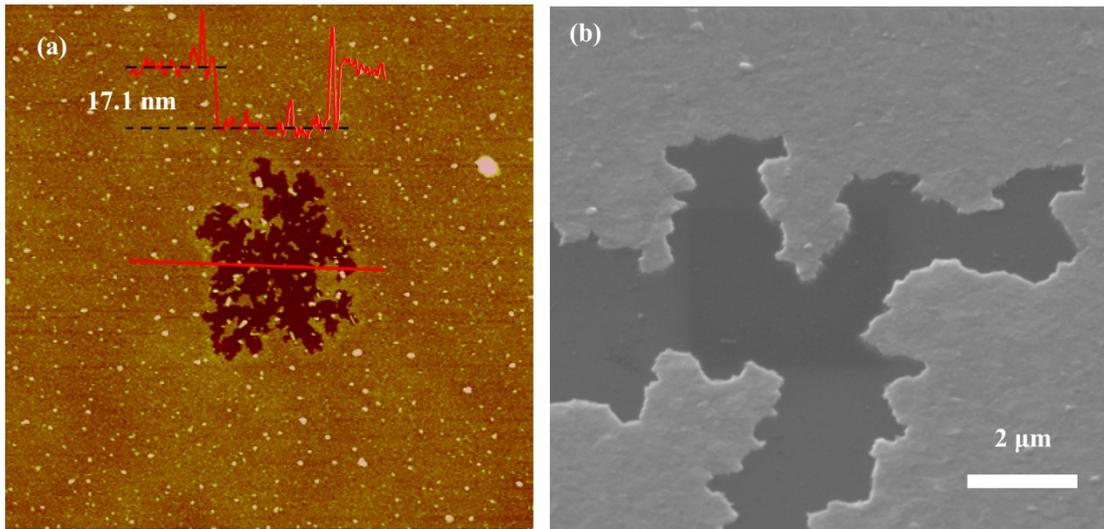
**Fig. S5 AFM and SEM images of annealed 2D  $\text{Bi}_{82}\text{Sb}_{18}$ .**
