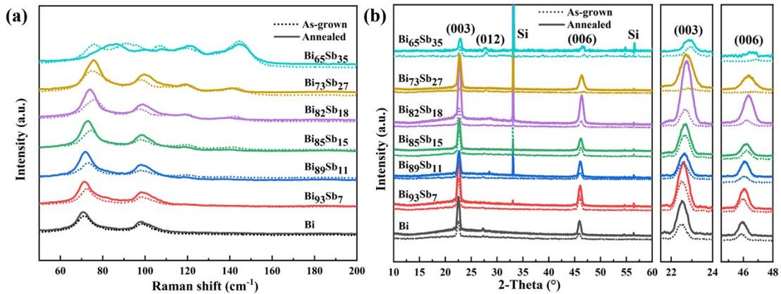
**Fig. S3** (a) XRD patterns and (b) Raman spectra of as-grown and annealed 2D bismuth antimonide
