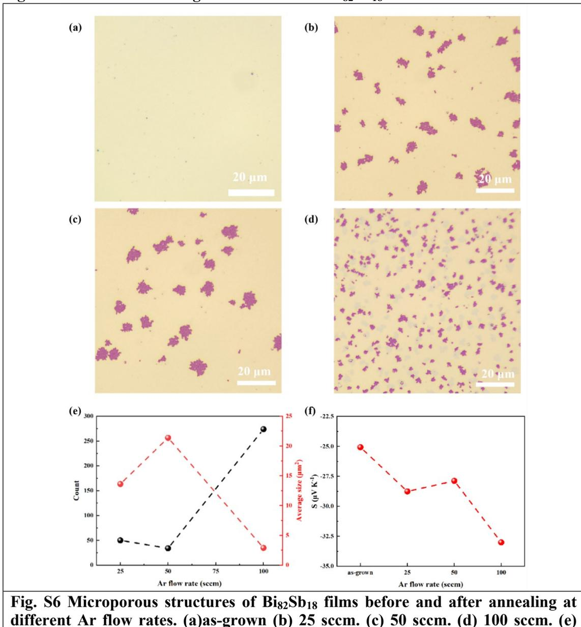
**Fig. S6 Microporous structures of  $\text{Bi}_{82}\text{Sb}_{18}$  films before and after annealing at different Ar flow rates. (a) as-grown (b) 25 sccm. (c) 50 sccm. (d) 100 sccm. (e)**
