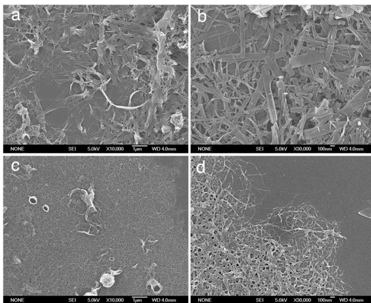
**Figure S9.** PANI-NF assembled with the assistance of aniline dimer. (a) and (b) SEM images of the assembled structure with a 60% PANI and 40% aniline dimer composition. (c) and (d) SEM images of the assembled structure with an 80% PANI and 20% aniline dimer composition.
