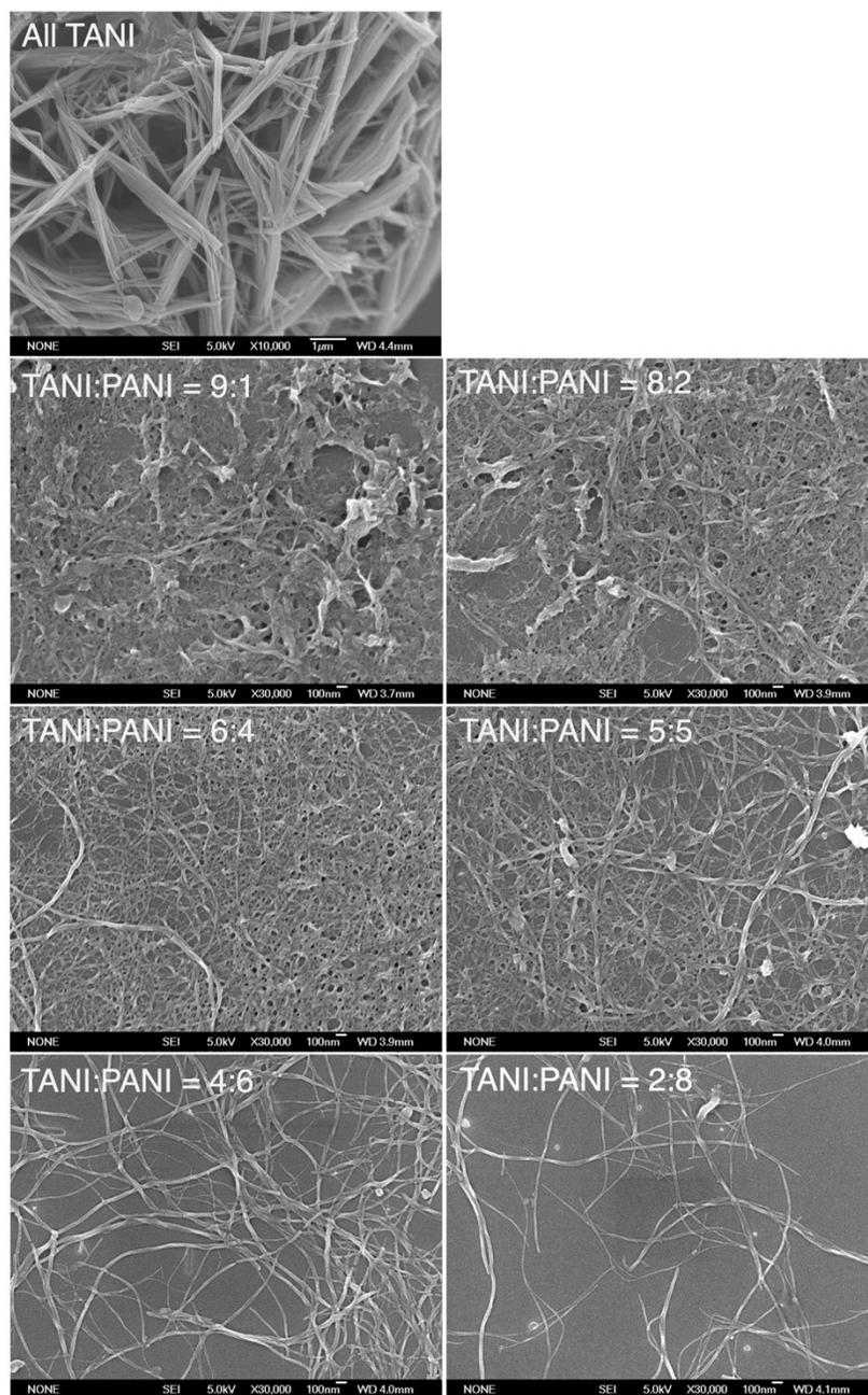
**Figure S5.** SEM images of TANI and TAS-PANI-NF self-assemble at different TANI:PANI ratio in a solvent mixture of 20% DMSO and 80% 0.1 M HClO<sub>4</sub>.
