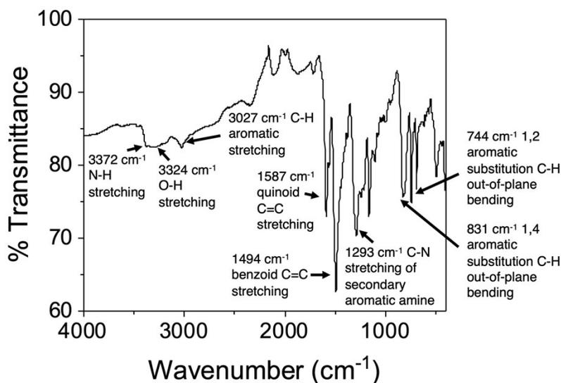
**Figure S1.** FT-IR spectrum with peak assignments of phenyl/amine-capped TANI.
