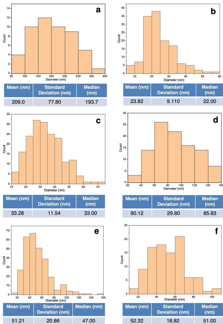
**Figure S4.** Diameter analysis of 20% TANI-assisted self-assembled nanostructures of PANI with defined molecular weight (Fig. 3): (a) 5,000 Da, (b) 10,000 Da, (c) 20,000 Da, (d) 50,000 Da, (e) 65,000 Da, (f) 100,000 Da.
