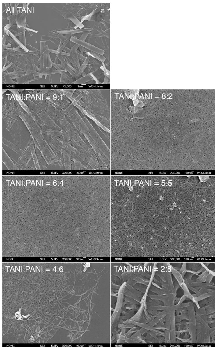
**Figure S6.** SEM images of TANI and TAS-PANI-NF self-assemble at different TANI:PANI ratio in a solvent mixture of 20% ethanol and 80% 0.1 M HClO<sub>4</sub>.
