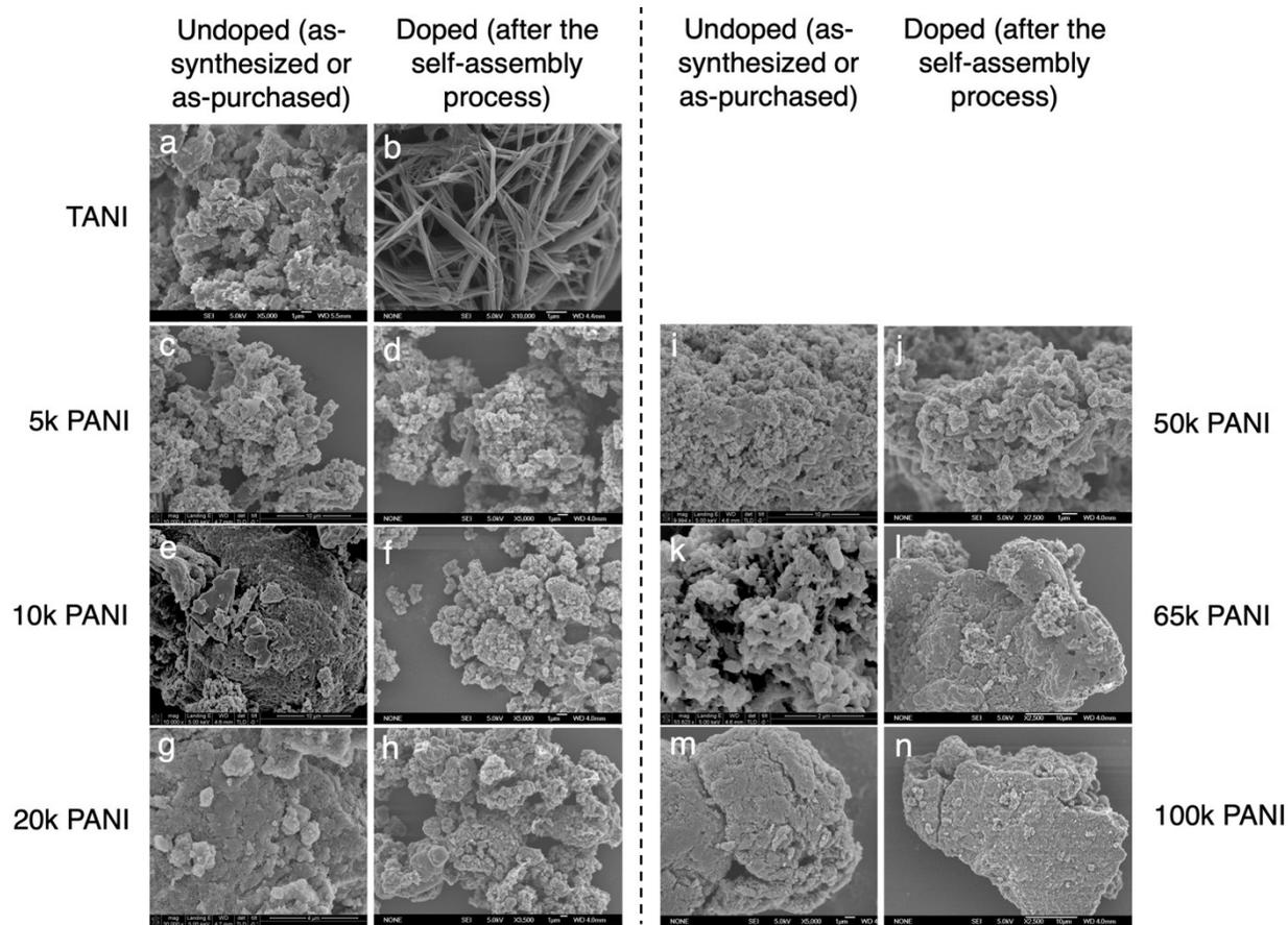
**Figure S7.** SEM images of TANI and PANI with various molecular weights in the as-synthesized (TANI) or as-purchased (PANI) forms vs. after self-assembly in a solvent mixture of either 20% THF and 80% water (the undoped columns) or 20% THF and 80% 0.1 M HClO<sub>4</sub> (the doped columns).
