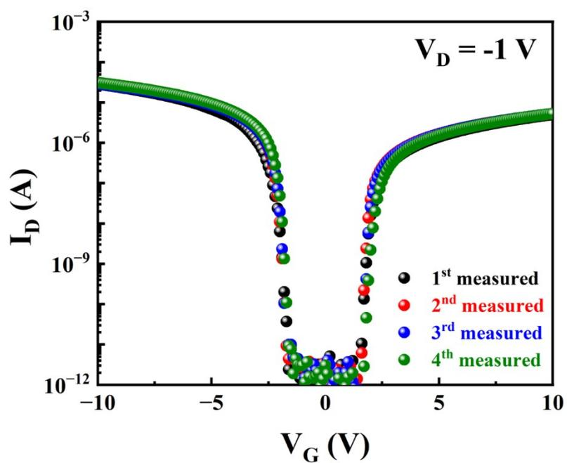
**Figure S3.** Repeated measurements used to build the transfer curve for the same SBT device.
