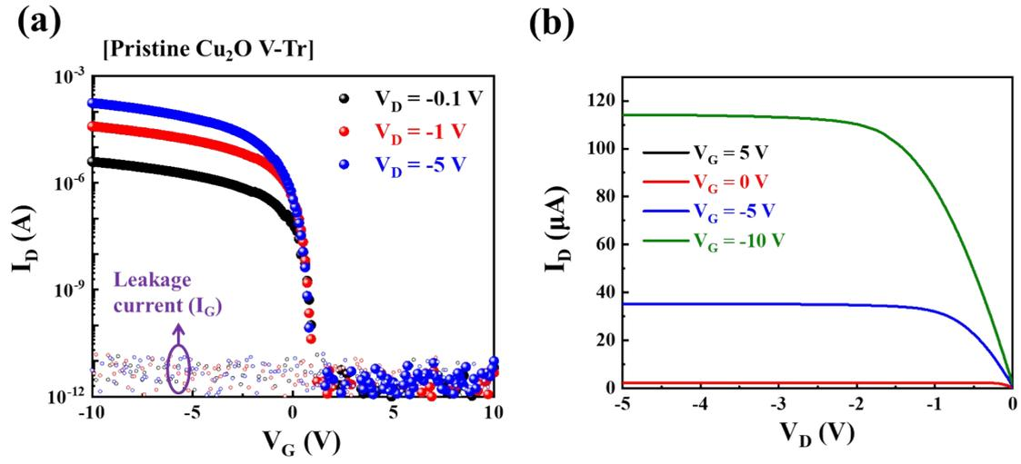
**Figure S2.** Electrical performances of OPT-free vertical  $p$ -type Cu<sub>2</sub>O transistor exhibiting unipolar characteristics: (a) Transfer and (b) Output curves.
