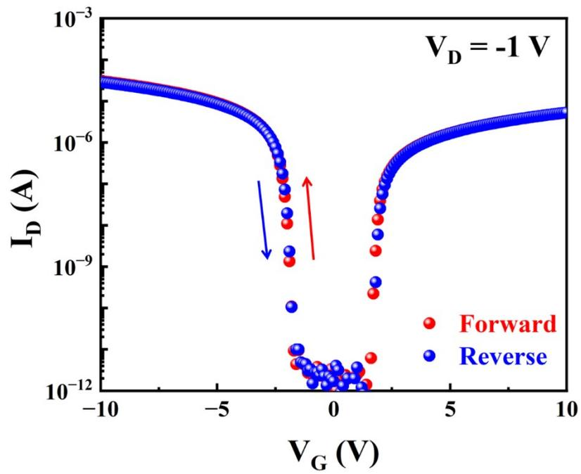
**Figure S4.** Hysteresis curve of an SBT device (500 nm thick  $\text{Cu}_2\text{O}$  layer) at  $V_D = -1$  V.
