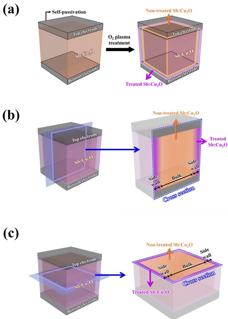
**Figure S6.** Schematic of a  $Cu_2O$  active layer used to evaluate the effect of  $O_2$  plasma treatment (a)  $Cu_2O$  active layer before and after treatment. Non-treated and  $O_2$ -plasma-treated regions along the (b) vertical and (c) horizontal directions. The non-treated and treated regions are shown in orange and purple, respectively.
