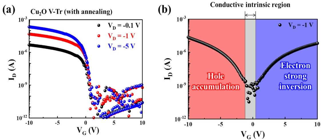
**Figure S1.** Electrical performances of vertical transistor device fabricated using high-conductivity *p*-type Cu<sub>2</sub>O channel. Transfer curves for (a) annealed and (b) annealed and OPT-treated transistors.
