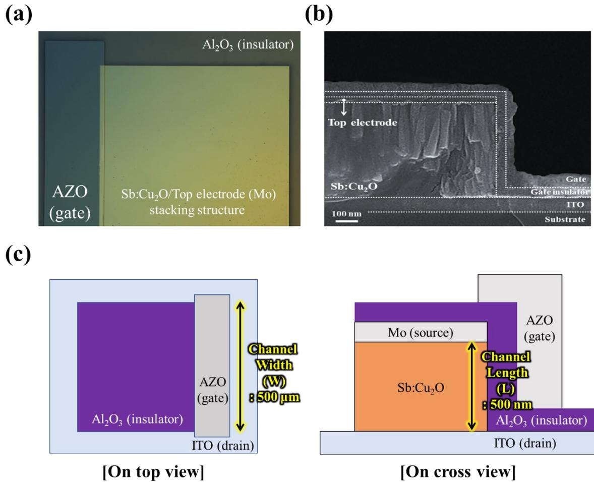
**Figure S5.** Structure and dimension of an SBT device: (a) optical micrograph, (b) cross-sectional SEM image, and (c) schematic of an SBT device including dimensions.
