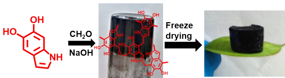
Figure S1. Schematic illustration of the aerogel fabrication strategy.
