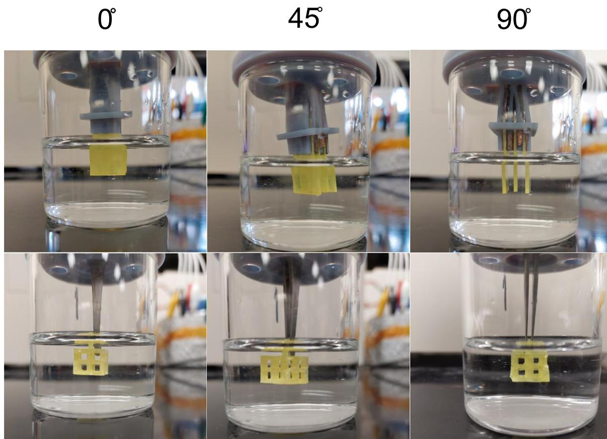
Fig. S5 Pictures of 3FG/ITO/Mo-BiVO<sub>4</sub> and 3DP/ITO/Mo-BiVO<sub>4</sub> electrode setup used for measuring the photocurrent density with varying illumination angle. The 0-degree orientation refers to when the flat glass surface is fully exposed to light, and a minimal exposure at 90 degrees illumination.
