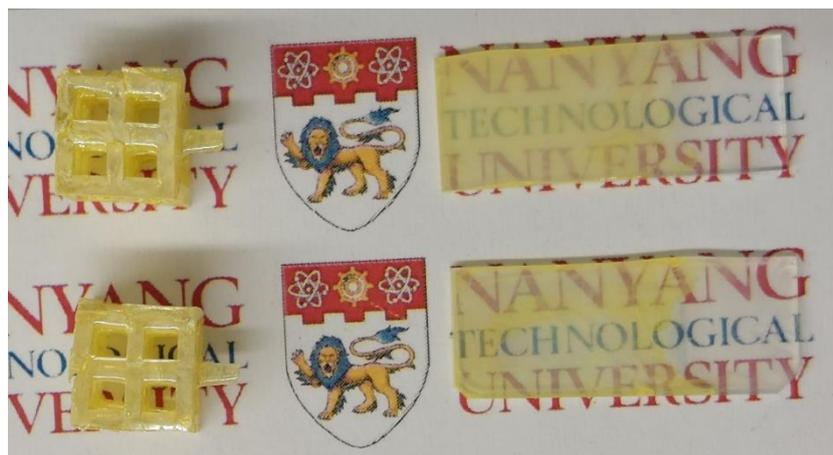
Fig. S2 Optical images of the 3D printed and glass substrates coated with ITO and Mo-BiVO<sub>4</sub>.
