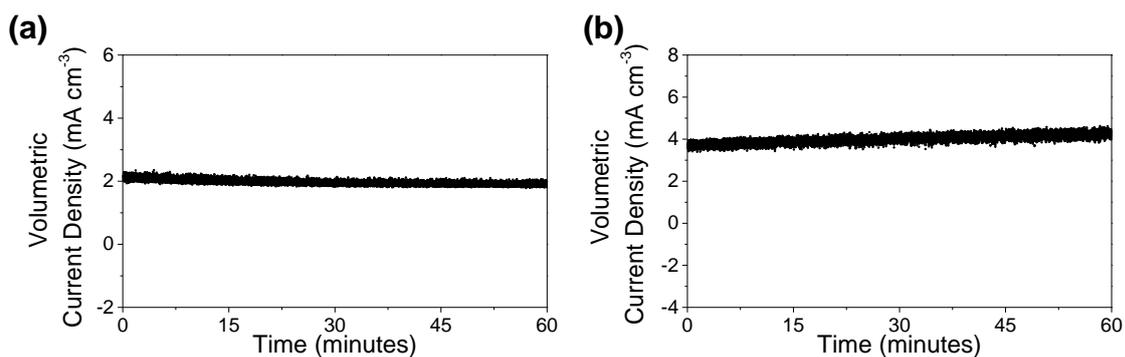
Fig. S7 Plot to investigate the variation of volumetric current density with time at 2 V for (a) 3FG sample, (b) 3DP (3\*3) lattice for 60 minutes. The test was conducted with constant stirring of the electrolyte in both cases.
