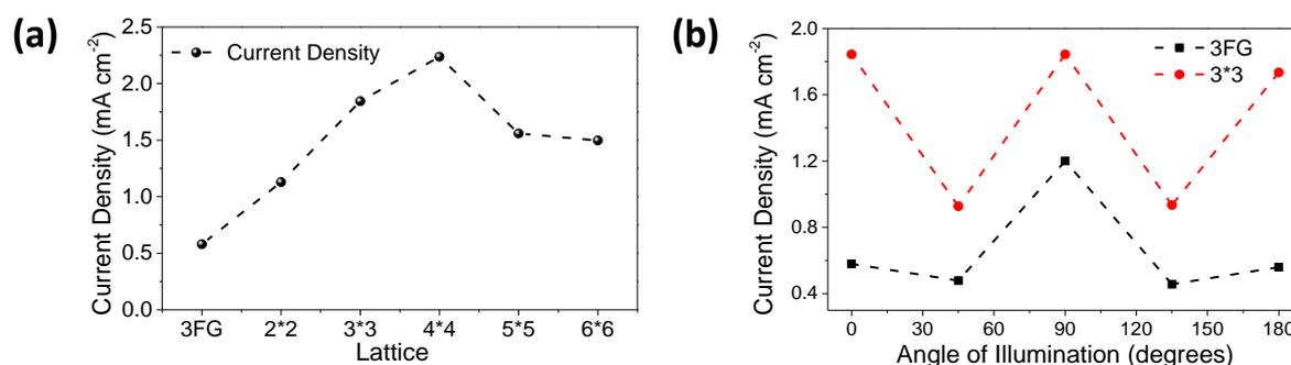
Fig. S9 (a) Comparison of current density based on orthogonally projected area at 1.23 V for various 3D printed lattices and 3FG sample, (b) plot of current density based on orthogonally projected area of 3D printed (3\*3) lattice and 3FG sample at 1.23 V at various angles of illumination.
