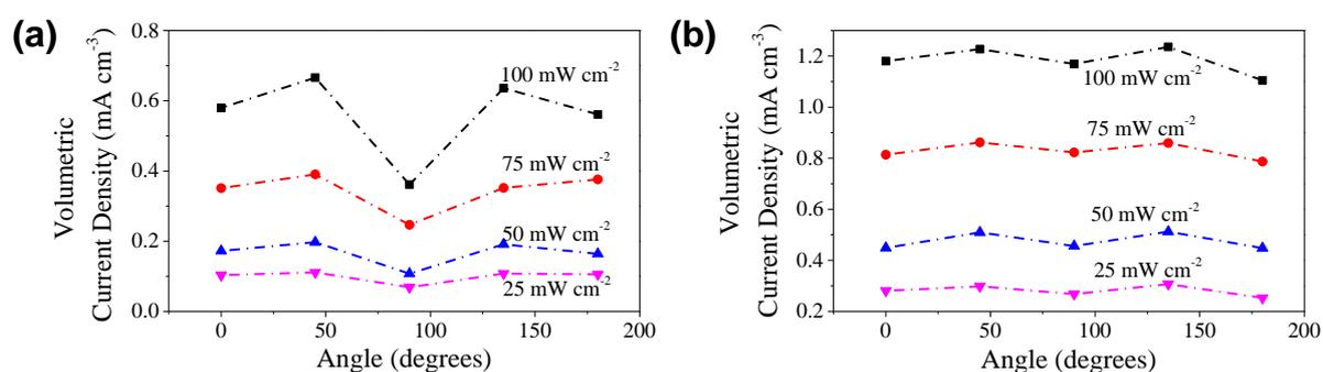
Fig. S6 Plot of volumetric current density vs angle of illumination at different light intensities for (a) 3FG sample, (b) 3D printed (3\*3) lattice.
