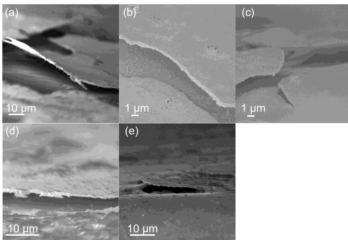
Fig. S1 FESEM cross section images of the (a) 2\*2, (b) 3\*3, (c) 4\*4, (d) 5\*5, and (e) 6\*6 lattices to estimate the approximate thickness of the ITO/BiVO<sub>4</sub> coating. Imaging of the cross-section view is difficult due to curved cross section of the cut glasses from the 3D lattice, hence the images of the flakes coming off the surface are taken to estimate the cross-section thickness.
