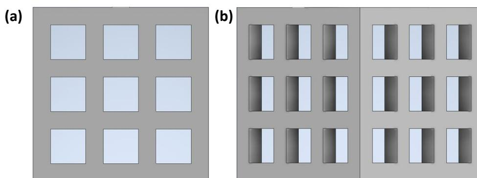
Fig. S8 Figure showing the orthogonal projected area of the 3D lattice (a) at 0 degrees, (b) at 45 degrees. The grey color represents the projected area and the blue color represents the excluded area.
