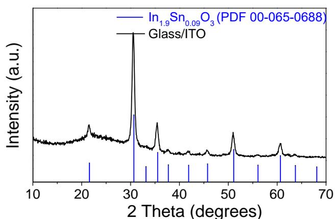
Fig. S3 X-ray diffraction spectra of Glass/ITO. (ITO here is the dip coated and annealed)
