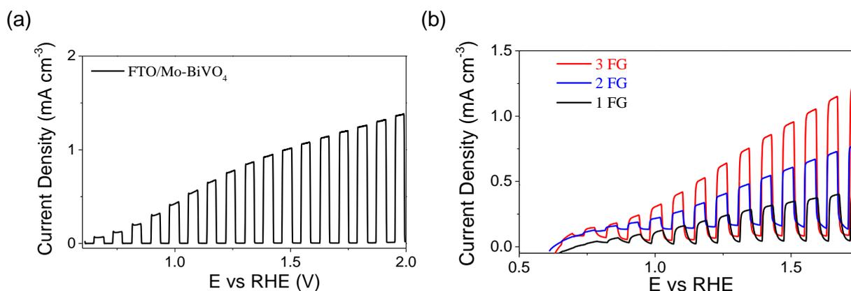
Fig. S4 Comparison of linear sweep voltammetry curves of (a) commercial FTO glass with dip coated Mo-BiVO<sub>4</sub> against, (b) different number of flat glass samples dip coated bifacially with ITO and Mo-BiVO<sub>4</sub> in series (assembled on behind another) for electrochemical water oxidation under chopped illumination. (1 FG refers to 1 flat glass sample and so on)
