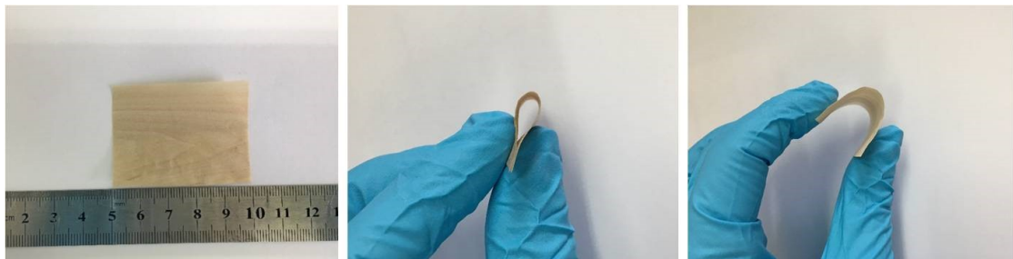
Fig. S2 Flexibility of a piece of modified wood film.
