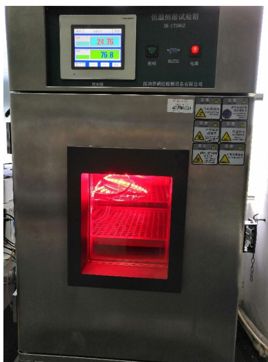
Fig. S30 A photograph of the device to measure impedance of sample after being illuminated by a red LED module.
