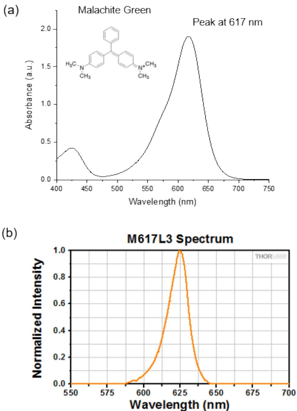
**Figure S3.** (a) Chemical structure and absorption spectrum of Malachite Green (MG) in water. (b) A spectrum of the visible LED with a nominal wavelength of 617 nm (THORLABS, M617L3) used to monitor the change of MG concentration in the photocatalytic degradation measurement. The spectrum was obtained from the THORLABS website.
