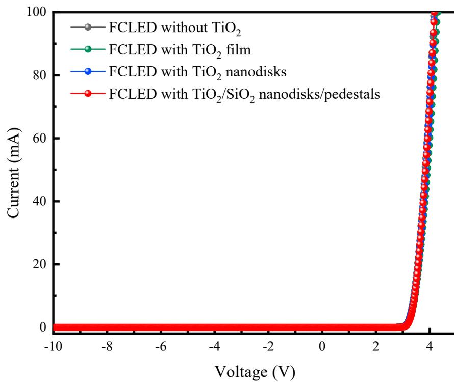
**Figure S5.** The current–voltage (I–V) characteristics of the near-UV LEDs with different TiO<sub>2</sub> nanostructures.
