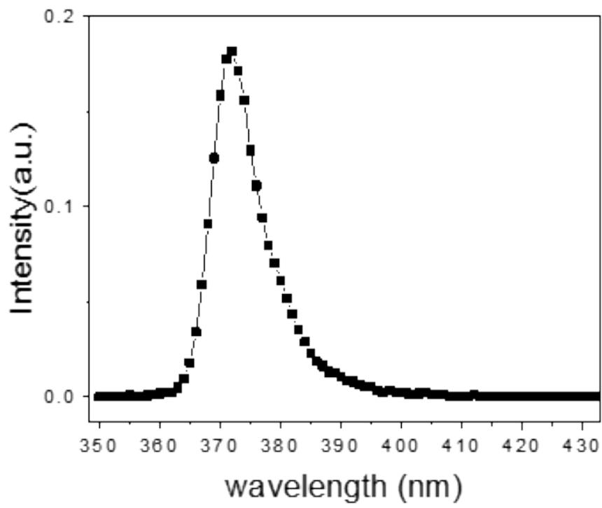
**Figure S1.** Spectrum of near-UV InGaN-based LED
