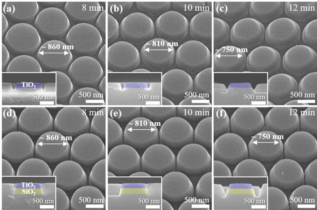
**Figure S4.** The bird's-eye view SEM images of (a-c) pristine TiO<sub>2</sub> nanodisk array and (d-f) TiO<sub>2</sub>/SiO<sub>2</sub> nanodisk/pedestal array as a function of the ICP etching time. Insets are the corresponding cross-sectional SEM images of nanodisks. As the ICP etching time increased, the diameter of the TiO<sub>2</sub> nanodisks gradually decreased.
