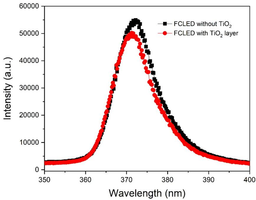
**Figure S7.** The light intensity measured from FCLEDs at the injection current of 20 mA. After application of TiO<sub>2</sub> layer, the extracted light intensity was decreased about 8.8%, which is probably attributed to the absorption of UV light by TiO<sub>2</sub> layer.
