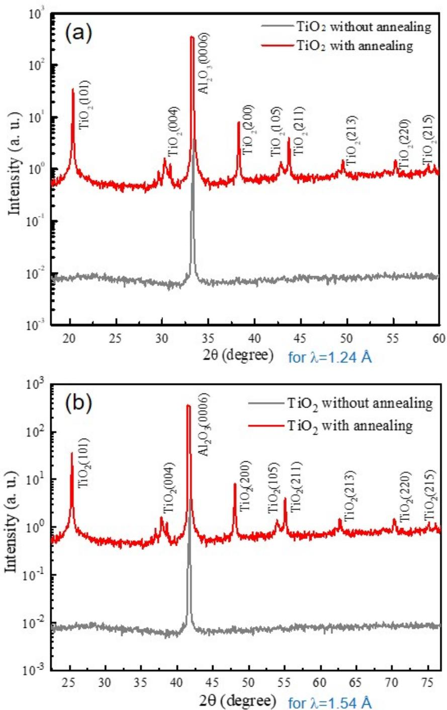
**Figure S6.** Indexing of XRD peaks. (a) A synchrotron X-ray source (1.24 Å) was used in our experiment. (B) The replotted XRD graph with the  $2\theta$  recalculated for the frequently used Cu  $K\alpha$  (1.54 Å) source for more convenient indexing of XRD peaks.
