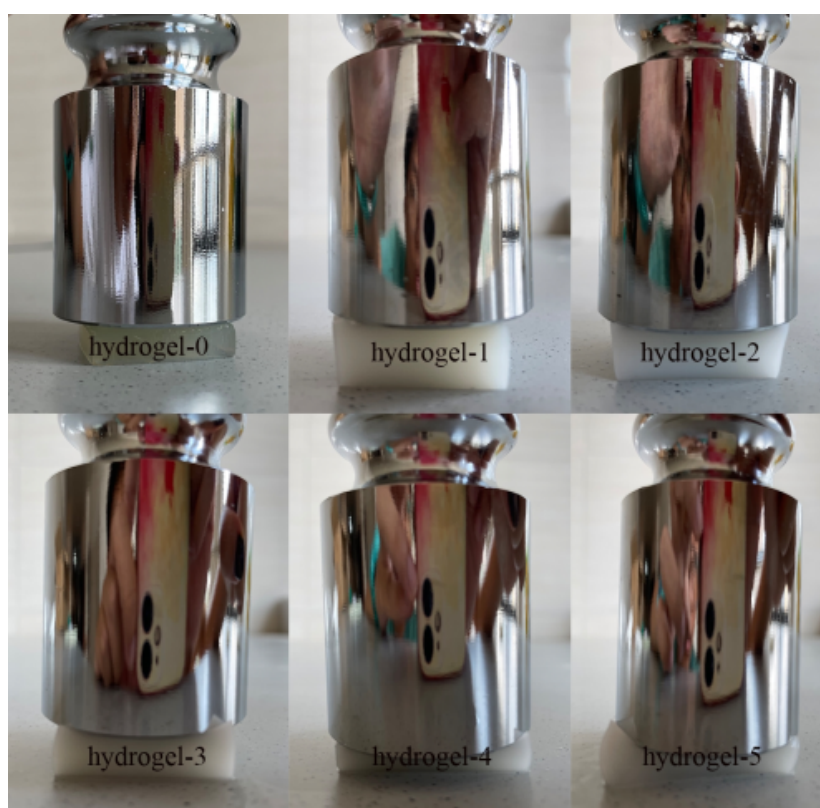
Figure S6. Under 500g weight, the degree of deformation of different hydrogels
