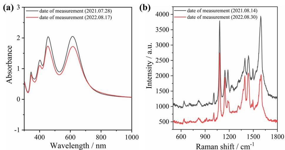
**Fig. S1** The (a) UV-Vis-NIR absorbance spectra and (b) SERS spectra of PATP under 633 nm excitation light of the Au@Ag core-shell nanorods after 1 year of storage.
