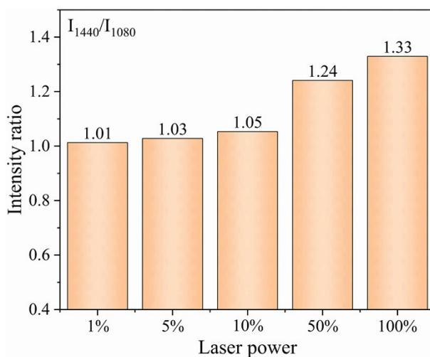
**Fig. S4** The conversion rates of PATP under the different power of 633 nm excitation light.
