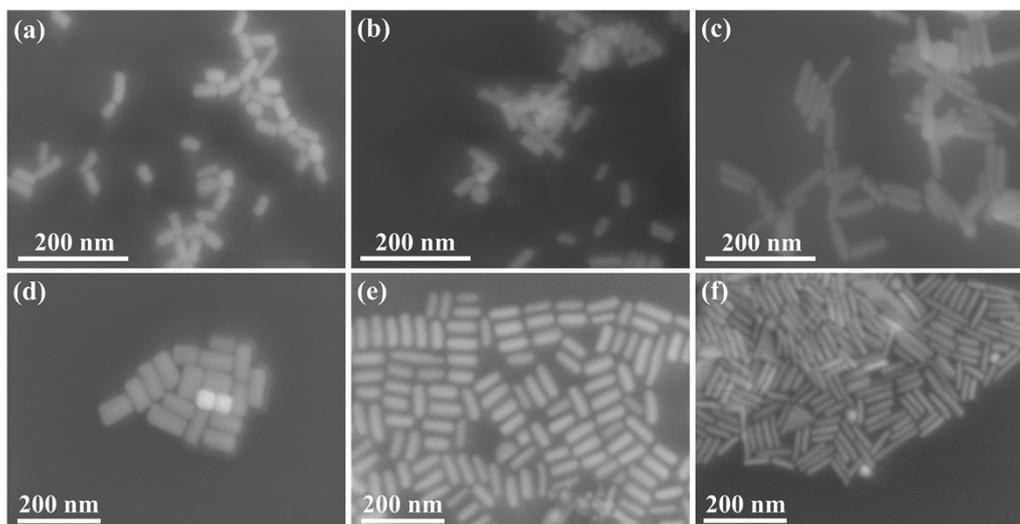
**Fig. S2** Au nanorods with different aspect ratios (a) 2.2, (b) 2.8, and (c) 4.2. Au@Ag core-shell nanorods with different aspect ratios (d) 1.8, (e) 2.7, and (f) 3.9.
