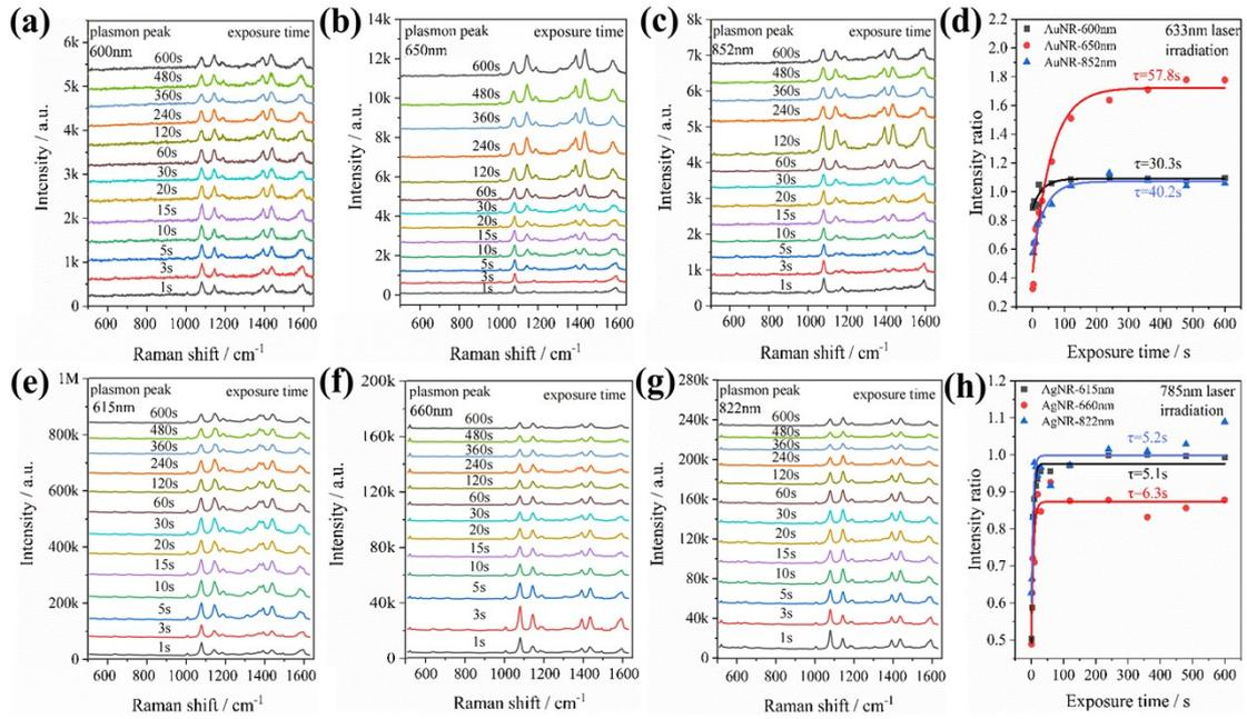
**Fig. S3** (a)-(c) Time-dependent SERS spectra of PATP adsorbed on Au nanorods and irradiated with 633 nm monochromatic light. (e)-(g) Time-dependent SERS spectra of PATP adsorbed on Au@Ag core-shell nanorods and irradiated with 785 nm monochromatic light. The variations of peak intensities at 1080 cm<sup>-1</sup> and 1440 cm<sup>-1</sup> with increasing irradiation time for (d) Au nanorods, (h) Au@Ag core-shell nanorods.
