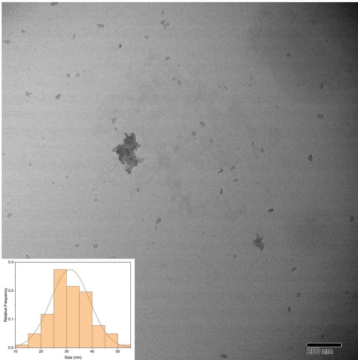
**Figure S2:** CNPs synthesized at 50 °C for 4 hours; TEM images: **a**, **b**, **c**; histogram: **d**, TEM image and histogram (inset, average size:  $31 \pm 8$  nm) of repetition experiment: **e**.
