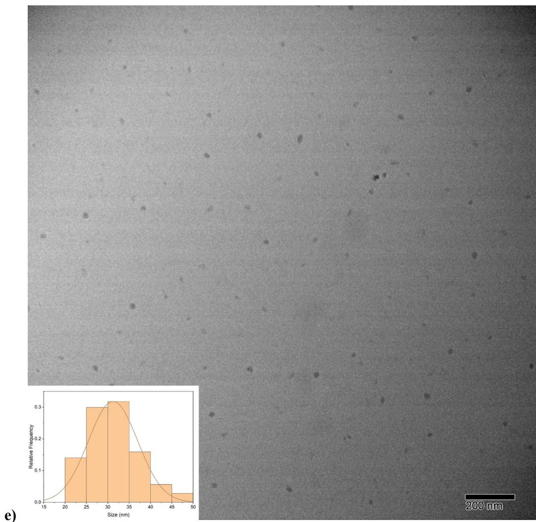
**Figure S1:** CNPs synthesized at 2;5 °C for 4 hours, TEM images: **a**, **b**, **c**; histogram: **d**, TEM image and histogram (inset, average size:  $31 \pm 6$  nm) of repetition experiment: **e**.
