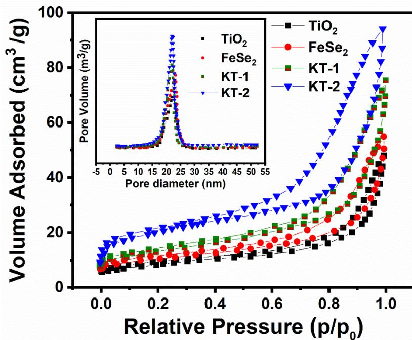
**Fig: S-1** The Brunauer-Emmett-Teller (BET) surface area was determined using nitrogen adsorption/desorption isotherms, and the insets show the associated pore-size distribution of the (a) TiO<sub>2</sub>, (b) FeSe<sub>2</sub> and (c) KT-1 and (d) KT-2 samples.
