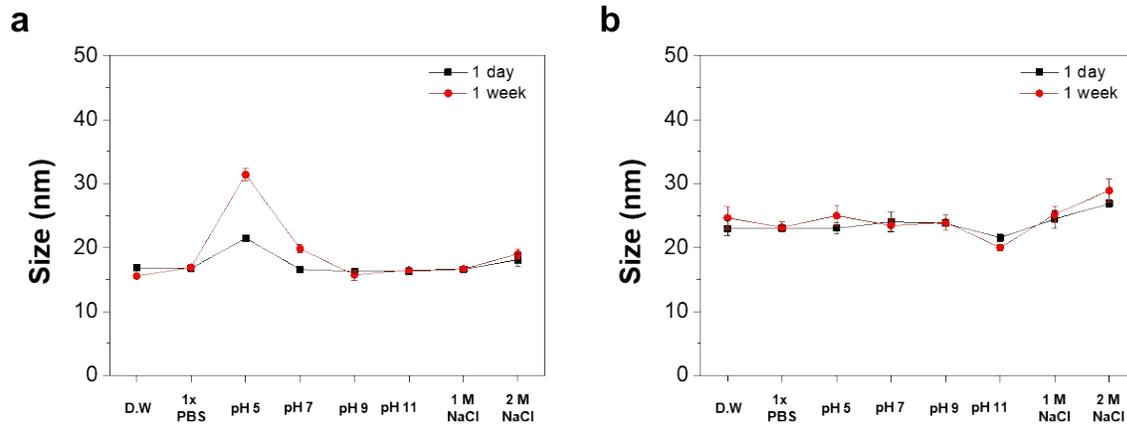
**Fig. S6** Stability measurement of MCP nanocoated (a) 8.5 nm and (b) 12 nm-sized IONPs by DLS in the wide range of pH and salt concentration.
