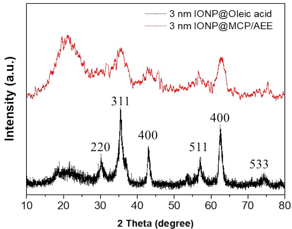
**Fig. S5** XRD patterns of 3 nm sized IONPs@Oleic acid and 3 nm sized IONP@MCP/AEE.
