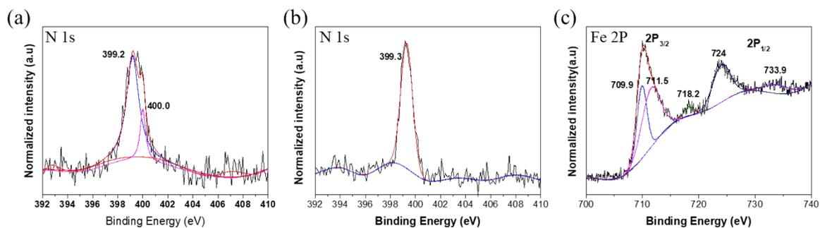
**Fig. S4** N 1s XPS spectra of (a) IONP@MCP/AEE and (b) MCP. (c) Fe 2P spectra of IONP@MCP/AEE.
