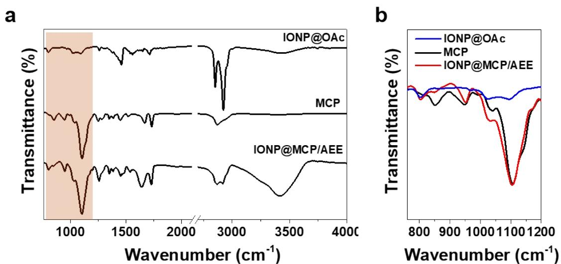
**Fig. S2** (a) FT-IR spectra of as-syn IONPs, MCP, and IONP@MCP/AEE and (b) enlarged FT-IR spectra of reddish boxed window of (a) spectra.
