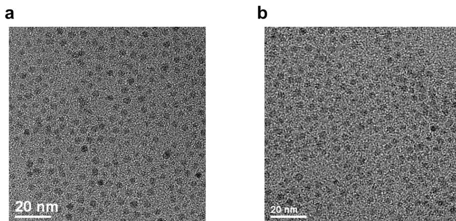
**Fig. S1** TEM image of (a) oleic acid capped 3 nm-sized IONPs, and (b) MCP coated 3 nm-sized IONPs by assistance of AEE.
