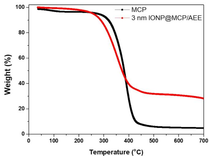
**Fig. S3** TGA data of 3 nm sized IONP@MCP/AEE and MCP.
