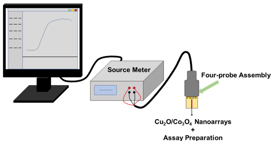
Fig. S1. Schematic sensing measuring system
