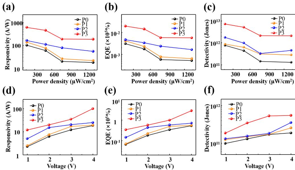
**Figure S11.** Photoresponsivity (a), EQE (b), and specific detectivity (c) of P0 and P1, P2, P3 devices under different light intensities and a voltage of 5 V. Photoresponsivity (d), EQE (e), and specific detectivity (f) of P0 and P1, P2, P3 devices with the light intensity of 19  $\mu\text{W}/\text{cm}^2$  under different voltages.
