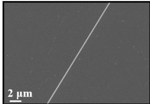
**Figure S1.** The SEM micrograph of CsPbBr<sub>3</sub> NW.
