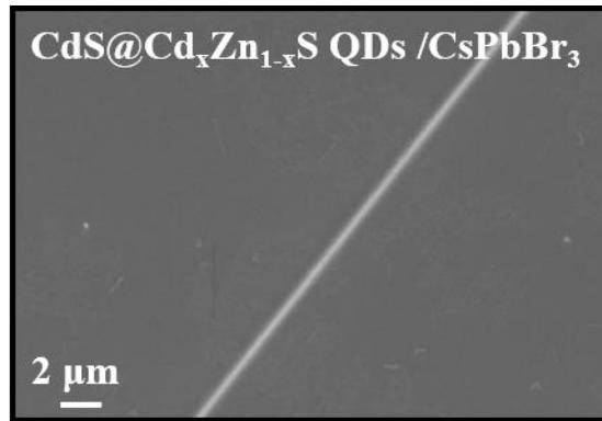
**Figure S3.** The SEM micrograph of  $\text{CsPbBr}_3$  NW after  $\text{CdS}@{\text{Cd}_x\text{Zn}_{1-x}\text{S}}$  QDs deposition.
