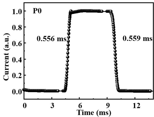
**Figure S6.** One cycle of the photoresponse under 405 nm laser at  $19 \mu\text{W}/\text{cm}^2$  for the P0 device.
