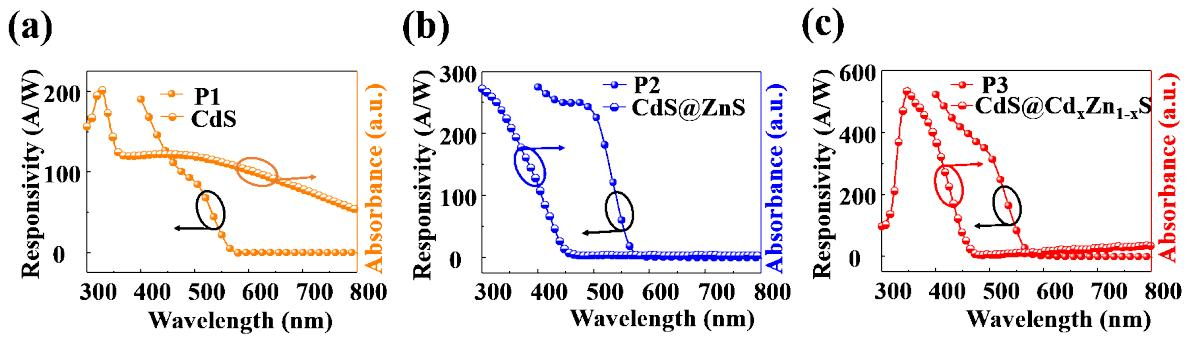
**Figure S8.** Photoresponsivity of P1, P2, P3 devices and the absorption curves of CdS QDs (a), CdS@ZnS QDs (b), CdS@Cd<sub>x</sub>Zn<sub>1-x</sub>S QDs (c) at wavelengths from 400 nm to 800 nm regions.
