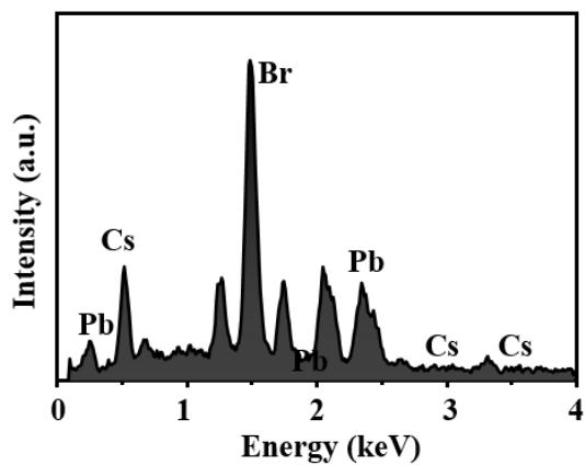
**Figure S2.** The EDS data of CsPbBr<sub>3</sub> NW.
