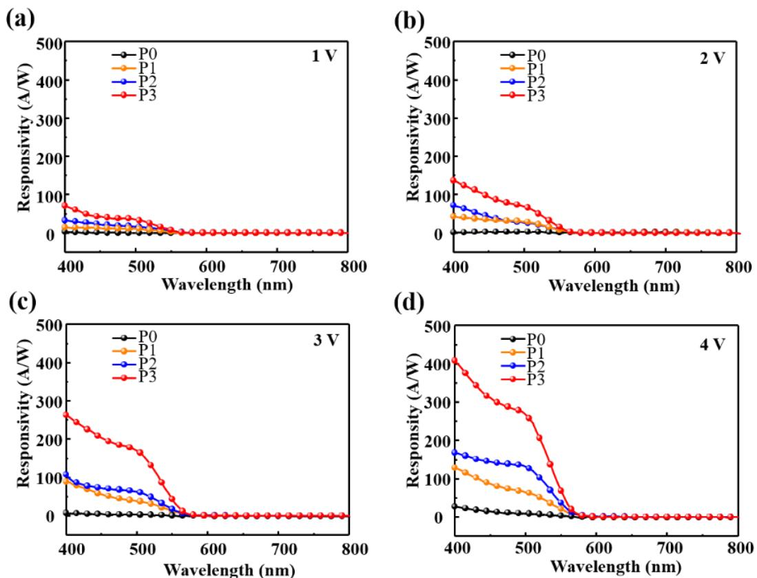
**Figure S9.** Photoresponsivity of P0, P1, P2, P3 devices at wavelengths from 400 nm to 800 nm regions under the increasing voltages of 1 V (a), 2 V (b), 3 V (c), and 4 V (d).
