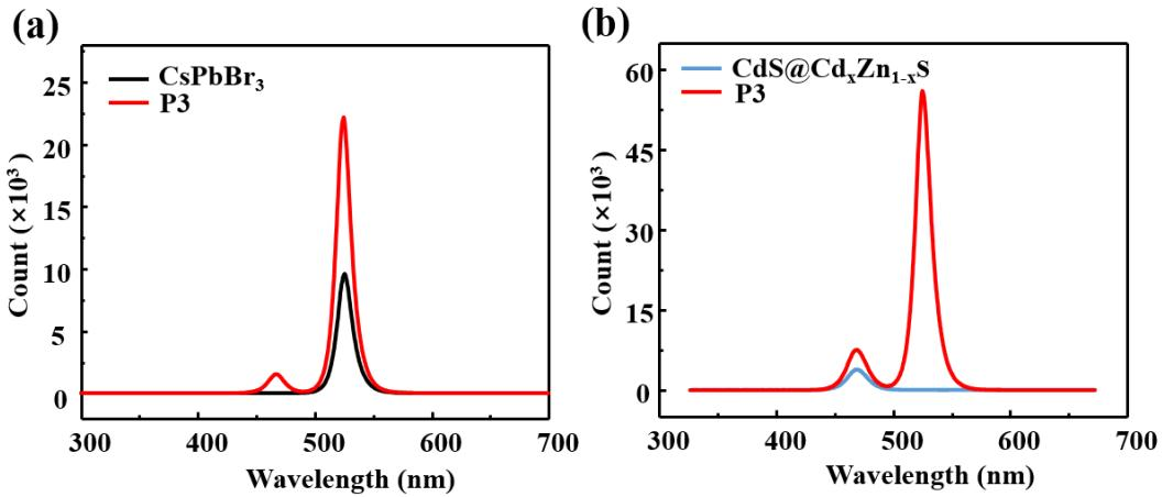
**Figure S10.** (a) The PL spectra of pure CsPbBr<sub>3</sub> NW and P3. (b) The PL spectra of pure CdS@Cd<sub>x</sub>Zn<sub>1-x</sub>S QDs and P3.
