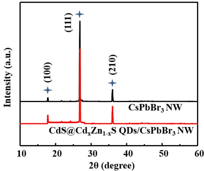
**Figure S5.** The XRD pattern of  $\text{CsPbBr}_3$  NW and  $\text{CdS}@{\text{Cd}_x\text{Zn}_{1-x}\text{S}}$  QDs/ $\text{CsPbBr}_3$  NW.
