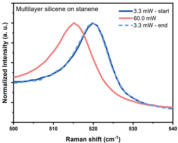
**Figure S4:** Normalized Raman spectra of the multilayer silicene on stanene/Ag(111) acquired at 3.3, at 60 and then again at 3.3 mW of laser power. The return of the Raman peak to its initial position demonstrates the absence of laser-induced structural changes.
