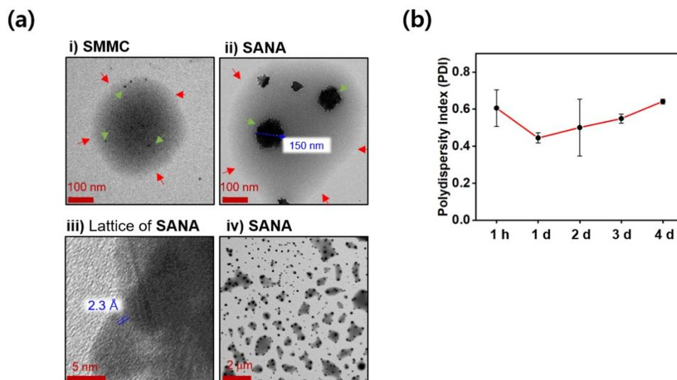
**Figure S2.** (a) TEM images coated by 1% (w/v) phosphotungstic acid (PTA) solution. i) SMMC. ii) Small-scale view of **SANA**. iii) Lattice of **SANA**. iv) Low magnification view of **SANA**. Red-color arrow: organic region. Green-color arrow: Au cluster region. (b) The polydispersity index (PDI) of **SANA** for 4 days in DI. H<sub>2</sub>O. The error bar represents the mean  $\pm$  S.D.
