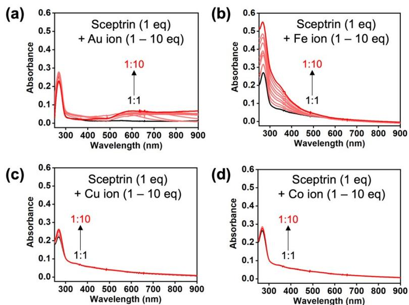
**Figure S1.** Absorption spectra of scep trin in the presence of metal ions (a)  $\text{AuCl}_3$ , (b)  $\text{FeCl}_2$ , (c)  $\text{CuCl}_2$ , (d)  $\text{CoCl}_2$  within DI  $\text{H}_2\text{O}$ . The measurement was conducted after 1 h incubation at 37 °C. The concentration of scep trin was 10  $\mu\text{M}$ . Tests were conducted in duplicate to obtain the measurements.
