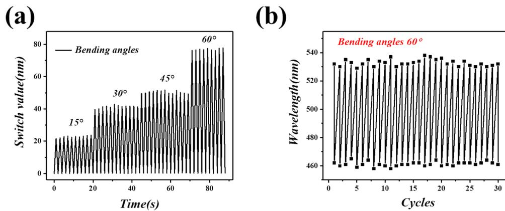
**Figure S4.** Durability test of hydrogel film bending cycles. (a) The wavelength shift values of the film in response to different bending angles. (b) Durability wavelength cycling test of structural color hydrogel film with bending angle of  $60^\circ$  .
