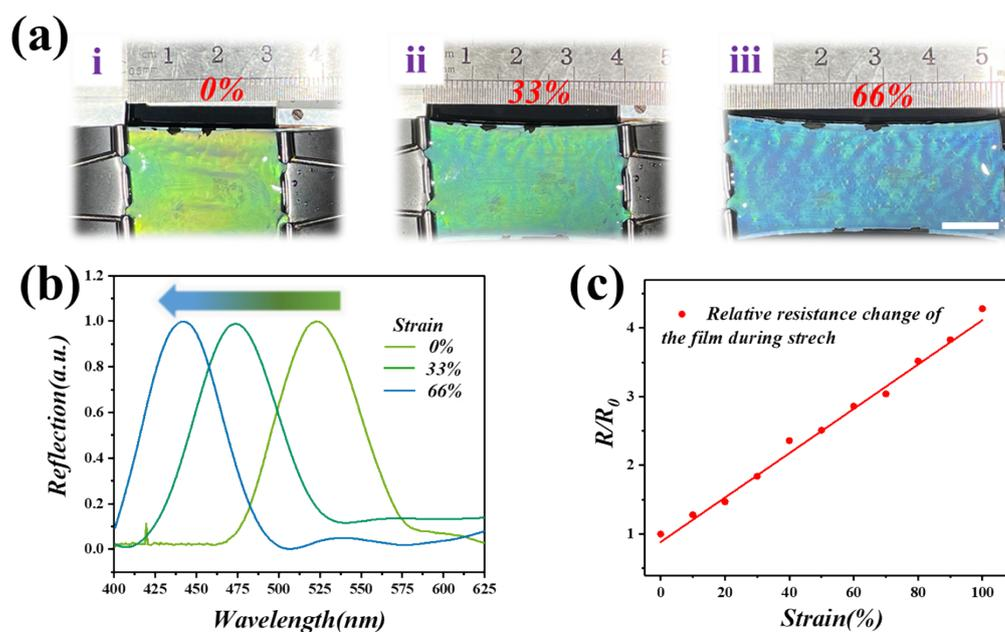
**Figure S1.** Optical image, spectral change and conductivity characterization of hydrogel structure during tensile process. (a) Color changes of inverse graphene films prepared by rGO doping P(NiPAAm-bis-AA) (2mg/mL) under different tensile conditions. (b) Reflection spectra under different tensile forces. (c) Change of relative resistance when the film is stretched. Scale bar is 1cm.
