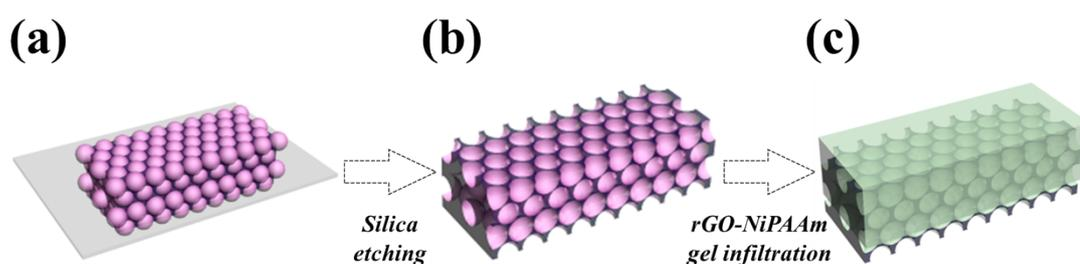
**Figure S3.** Preparation scheme of hydrogel film. Schematic diagram of generation process of polymer-conductive hydrogel hybrid color film.
