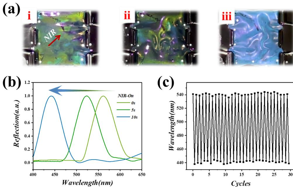
**Figure S2.** Optical properties and stability Characterization of hydrogel on NIR. (a)
