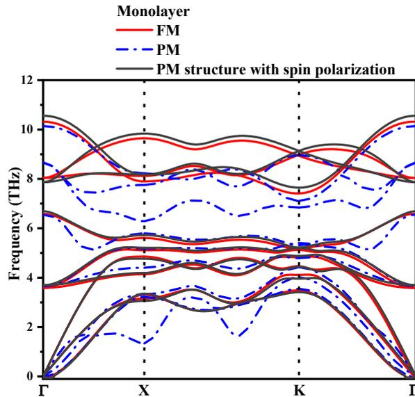
**Fig. S6** Phonon dispersion of monolayer FM phase (red lines), PM phase with (black lines) or without spin polarization (blue dotted lines). The phonon dispersion of PM structure with spin polarization is similar to that of FM structure but much different to that of PM structure without spin polarization, indicating that the large thermal conductivity variation in 2H-VSe<sub>2</sub> is caused by magnetic order while structural change has weak effects.
