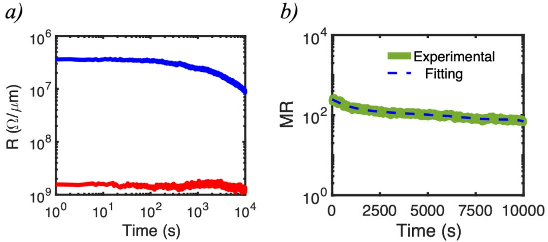
**Supporting Figure S8:** a) A 2D plot for long term retention of two representative analog resistance states for an extended period of time approximately  $10^4$  seconds or roughly 3 hours. b) A plot of memory ratio (MR) between the two states with time. MR varied from  $3 \times 10^2$  to  $1 \times 10^2$  with an exponential decay time
