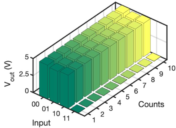
**Supporting Figure S7:** Normal NAND functionality observed for a  $V_{DD} = 5V$  despite the presence of HT at the rare node ( $V_{DD} = 2V$ ).
