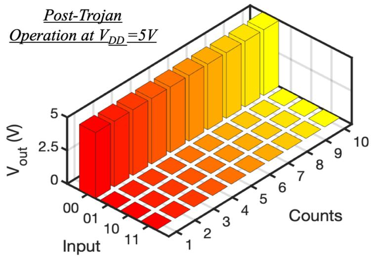
**Supporting Figure S6:** Normal *NOR* functionality observed for a  $V_{DD} = 5V$  despite the presence of HT at the rare node ( $V_{DD} = 2V$ ).
