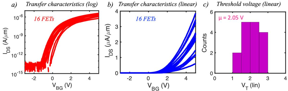
**Supporting Figure S1:** Evaluating device-to-device variation across a population of 16 MoS<sub>2</sub>-based FETs by measuring the transfer characteristics in a) logarithmic scale and b) linear scale. The devices consistently show good  $I_{ON}$  values with  $I_{ON}/I_{OFF}$  ratios of about  $10^7$ . c) A histogram plot of the threshold voltage ( $V_{TH}$ ) extracted from the linear scale once again prove the high quality of MOCVD grown MoS<sub>2</sub>.
