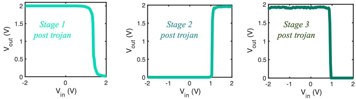
**Supporting Figure S5:** The corresponding output inverter plots post  $V_{HRT}$  application of 15 V to one of the local gates  $MT2$  from stage 1. A clear shift in the switching voltage  $V_m$  is observed for all the stages.
