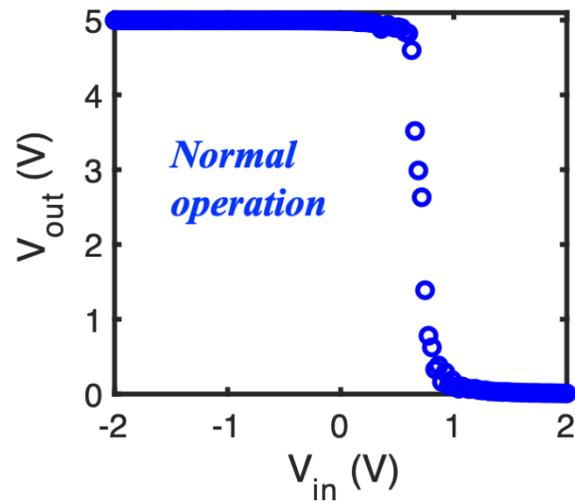
**Supporting Figure S3:** Inverter output characteristics for a supply voltage  $V_{DD} = 5V$ . The inverter shows normal characteristics at higher supply voltage in spite of the presence of a HT at lower  $V_{DD} = 2V$ .
