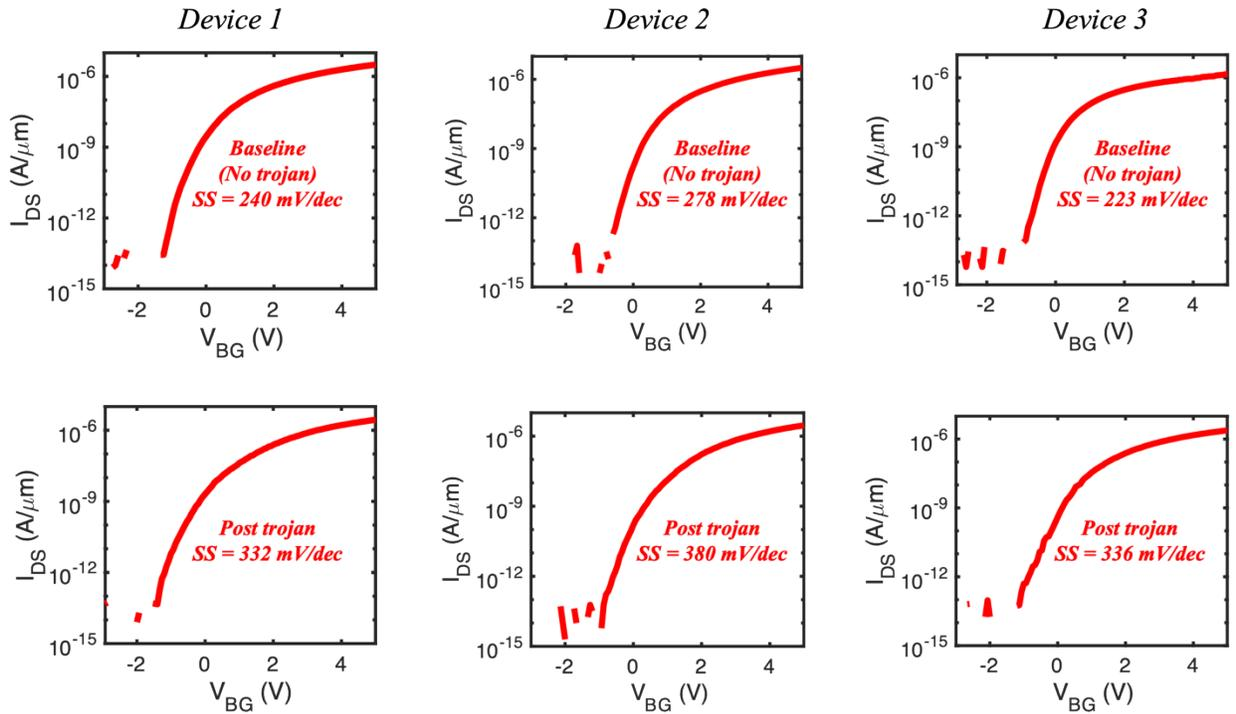
**Supporting Figure S4:** Evolution of degradation observed in the subthreshold slope (SS) of a 2D memtransistor in a cascaded three-stage inverter (TSI) circuit module as a form of HT for three different individual MoS<sub>2</sub> memtransistors post application of a  $V_{HRT}$  of 15V followed by a  $V_{LRT}$  of -15V to the local gates.
