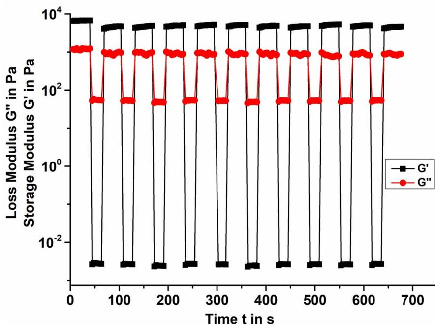
**Fig. S7:** Rheological recovery behaviors of DZC hydrogel with multiple cycles. (Black and red curves display storage and loss modulus, respectively.)
