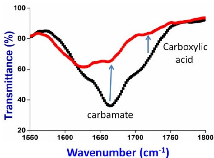
**Fig. S9:** FTIR spectra of tryptophan-induced hydrogel, without UV-exposure (black) and with UV-exposure (red).
