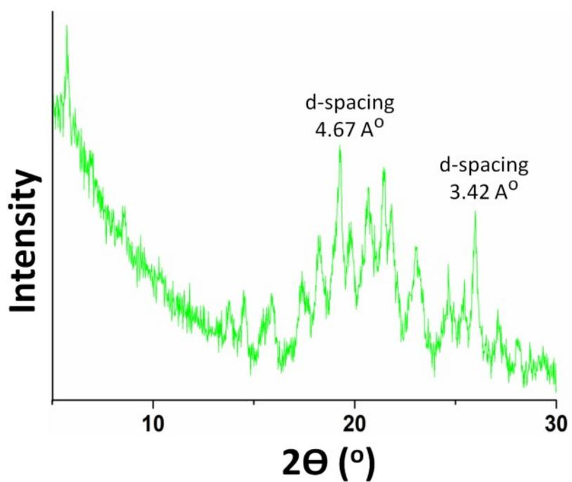
**Fig. S6:** The wide-angle X-ray scattering (WAXS) patterns of the powder ZDC.
