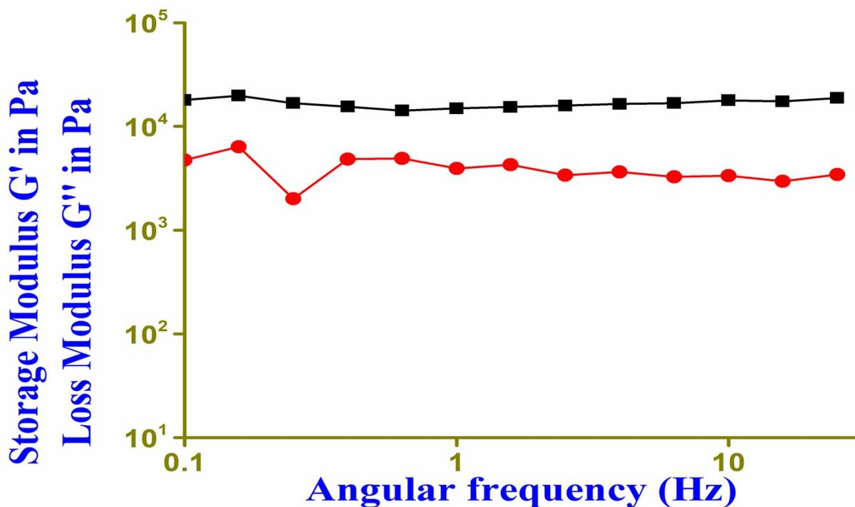
Fig. S3: Frequency-sweep experiment of DZC gel at a constant strain of 0.01%.
