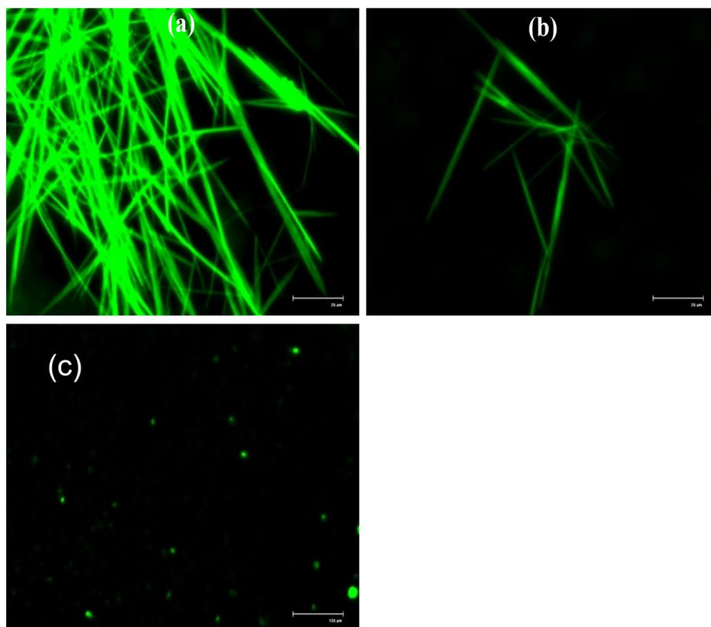
**Fig. S13:** Fluorescence microscopy images of the DZC and tryptophan-induced hydrogel, (a) before, (b) after exposure to UV light and (c) only with Th T (control).
