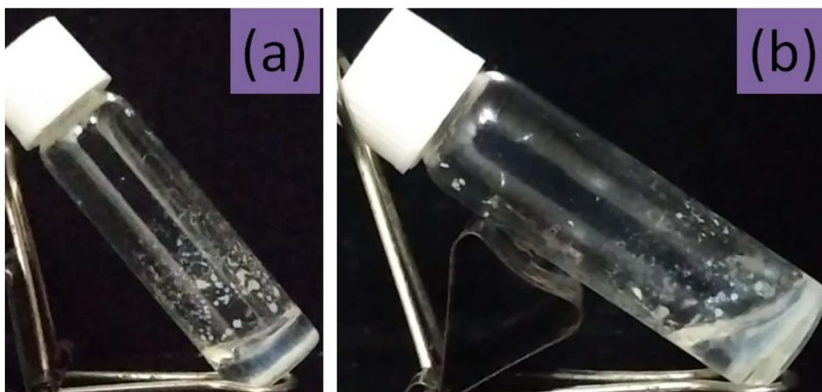
**Fig. S8:** Vial image of tryptophan-induced hydrogel, (a) without UV-exposure and (b) with UV-exposure.
