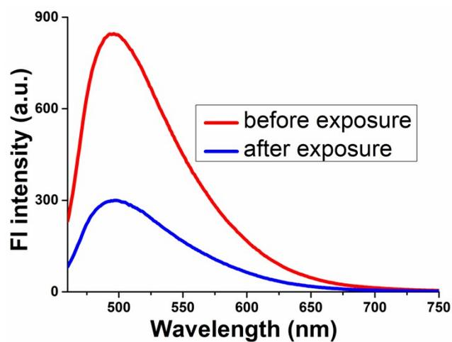
**Fig. S12:** Th T fluorescence spectra of the DZC and tryptophan-induced hydrogel before (red) and after (blue) exposure to UV light. The excitation wavelength was 450 nm, and the concentration of Th T was 8  $\mu$ M.
