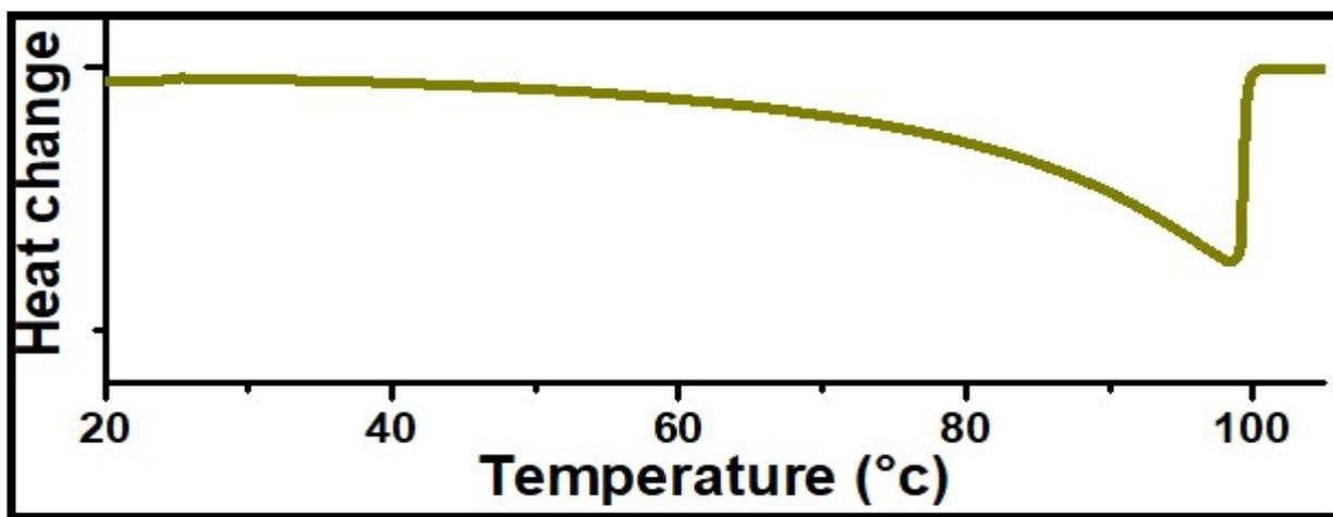
Fig. S4: DSC thermograms of ZDC hydrogels prepared at gelator concentration: 6.5 g/L. The  $T_{DSC} = 98\text{ }^{\circ}\text{C}$  at gelator conc. 6.5 mg/mL.
