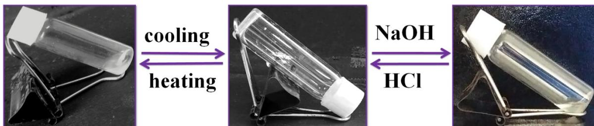
Fig. S1: Temperature and pH-responsive nature of the hydrogel.
