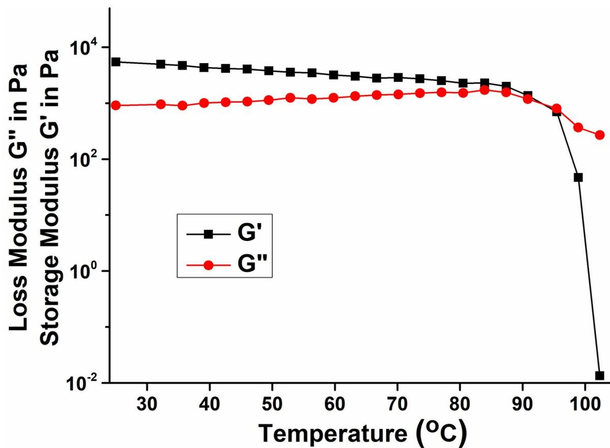
Fig. S2: temperature dependant rheology experiment of ZDC hydrogel.
