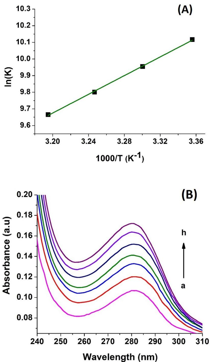
**Fig. S4.** Van't Hoff plot for the OVA-5-CQA system (A), UV-Vis absorption spectra of OVA ( $5.00 \times 10^{-6} \text{ mol dm}^{-3}$ ) in the presence of various concentrations of C- $\text{Fe}_3\text{O}_4$  NPs at 298 K (B), [OVA]:  $= 5.00 \times 10^{-6} \text{ mol dm}^{-3}$ ; [C- $\text{Fe}_3\text{O}_4$  NPs]: [a-i]: 0.00, 0.40, 0.80, 1.20, 1.60, 2.00, 3.00, 4.00 and  $5.00 \times 10^{-6} \text{ mol dm}^{-3}$ .
