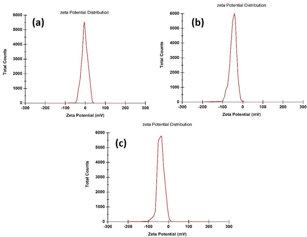
**Fig. S2.** The Zeta potential distribution of Fe<sub>3</sub>O<sub>4</sub> NPs (a), C-Fe<sub>3</sub>O<sub>4</sub> NPs (b) and C-Fe<sub>3</sub>O<sub>4</sub> NPs@OVA (c)
