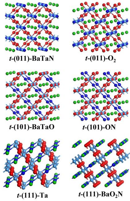
**Fig. S1** Slab models of (011), (101) and (111) surfaces for *trans*  $\text{BaTaO}_2\text{N}$ . The green, light blue, red, and dark blue balls represent Ba, Ta, O, and N atoms, respectively.
