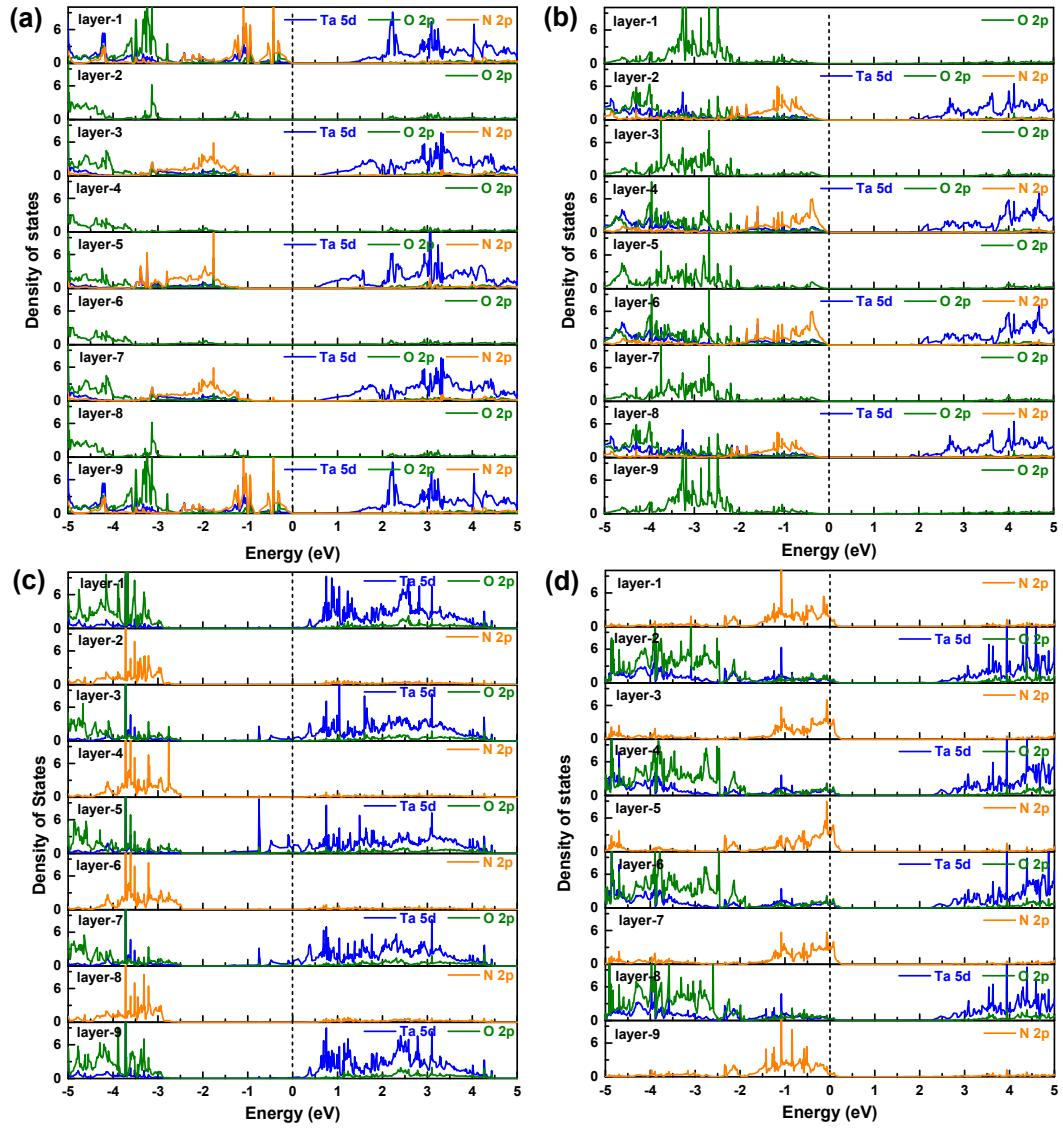
**Fig. S2** The layer-resolved spin-up density of states for (a)  $t$ -(001)-TaON, (b)  $t$ -(001)-BaO, (c)  $t$ -(100)-TaO<sub>2</sub>, and (d)  $t$ -(100)-BaN.
