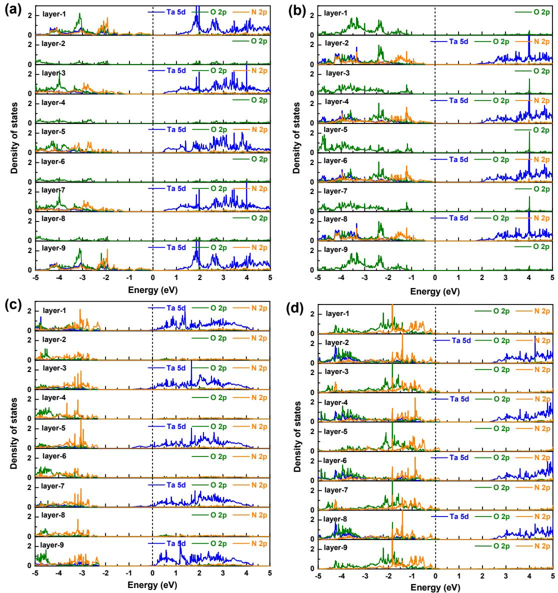
**Fig. S3** The layer-resolved spin-up density of states for (a) *c*-(001)-TaON, (b) *c*-(001)-BaO, (c) *c*-(100)-Ta<sub>2</sub>O<sub>3</sub>N, and (d) *c*-(100)-Ba<sub>2</sub>ON.
