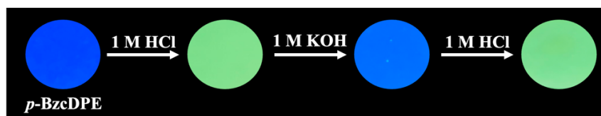
Fig. S11. Regeneration of p -BzcdPE pre-stained filter paper under UV light (365 nm).
