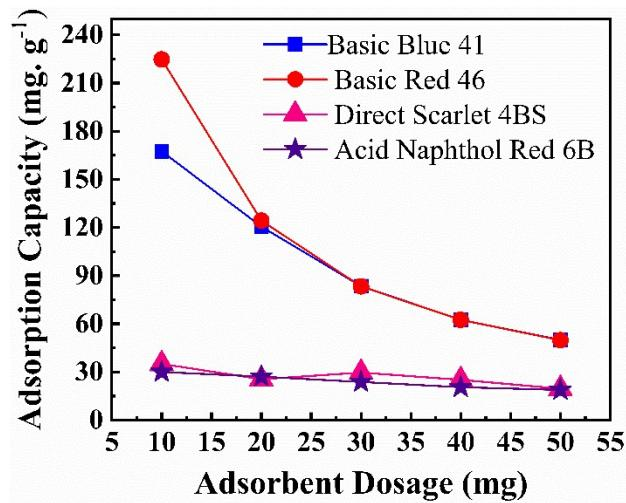
Figure 3s. Effect of adsorbent dosage on the adsorption capacity.
