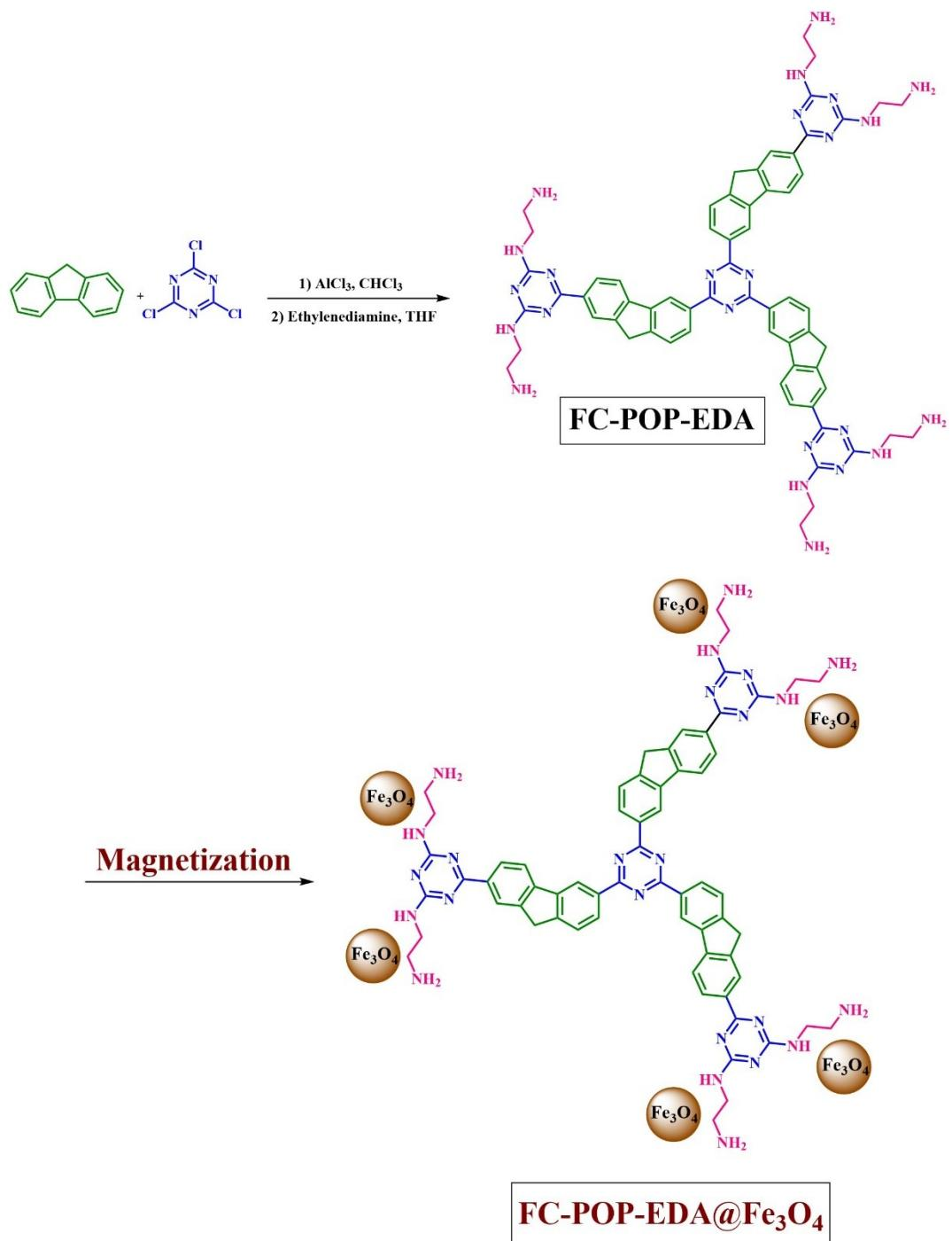
Figure 1s. Synthetic scheme of POP modification with EDA and Fe<sub>3</sub>O<sub>4</sub>.
