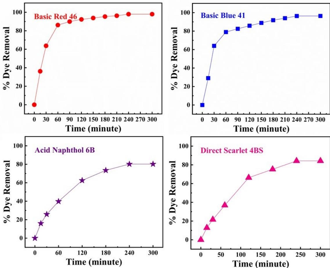
Figure 4s. Adsorption percentage of dyes versus contact time.
