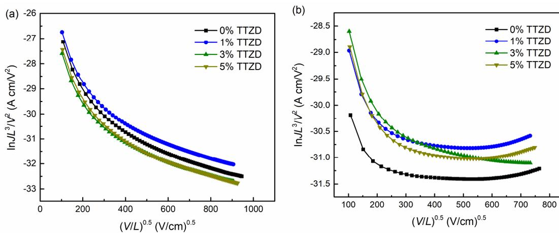
**Figure S5.**  $J$ - $V$  curves fitted by the SCLC method for hole- (a) and electron-only (b) devices.
