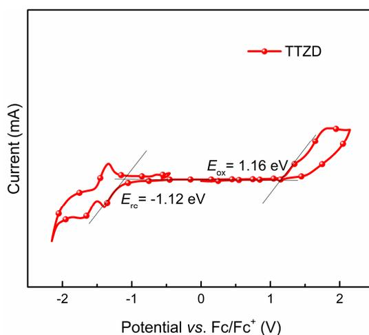
**Figure S4.** Cyclic voltammetry (CV) curves of TTZD.
