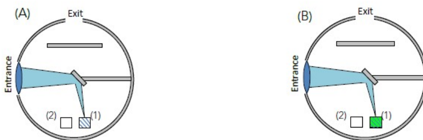
Figure 1. Two different measurement configurations required for Direct Excitation measurements: (A) reference sample (solvent only) in sample position (1); (B) test sample in position 1 (position 2 remains empty for both measurements.)
