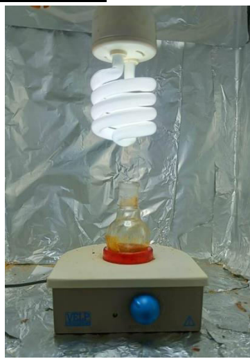
Figure. 20 W CFL bulb utilized for the photochemical reaction
