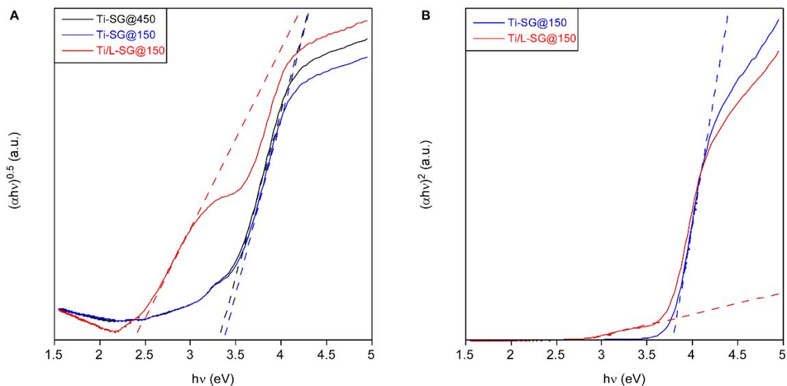
**Fig. S3** Tauc plots of coatings cured at 150 and 450 °C. Dashed lines depict the linear fitting of (A)  $(\alpha h\nu)^{0.5}$  for the indirect band gap and (B)  $(\alpha h\nu)^2$  for the direct band gap.
