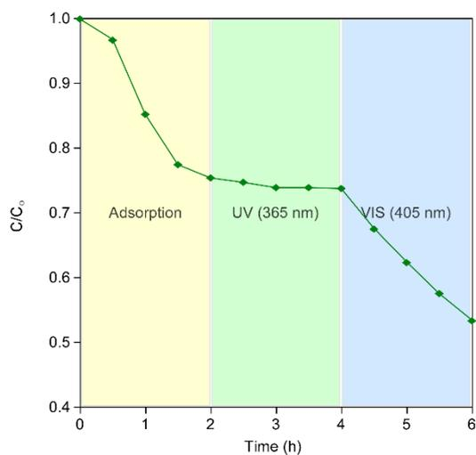
**Fig. S6** Evolution of the relative dye concentration using UV light illumination prior to visible irradiation for Ti/L-SG@150.
