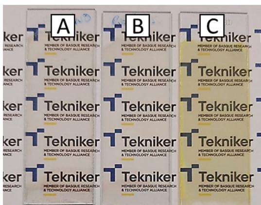
Fig. S2 Coatings appearance of coated glass supports: (A) Ti-SG@450, (B) Ti-SG@150 and (C) Ti/L-SG@150.
