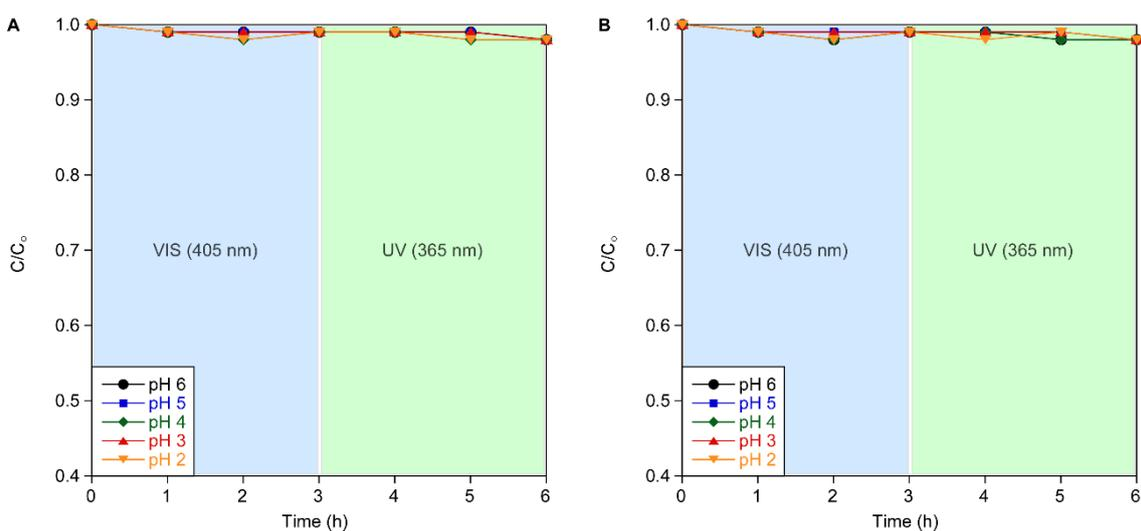
**Fig. S4** Evolution of the relative dye concentration under visible and UV light (A) in absence of substrate and photocatalyst and (B) in presence of the substrate without photocatalyst.
