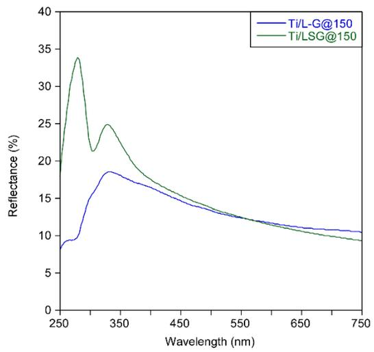
**Fig. S7** Comparison of reflectance spectra of Ti/L-SG@150 and Ti/L-G@150.
