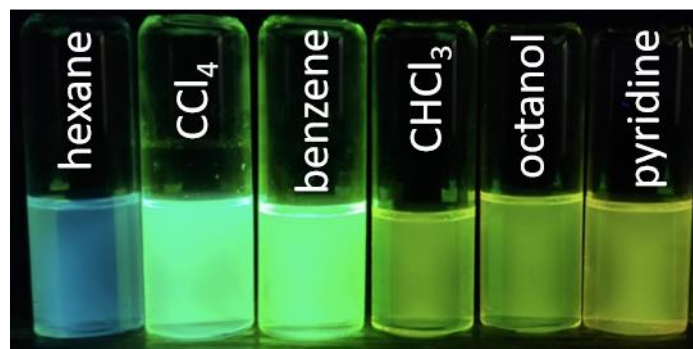
Fig. S13 Molecule 1 at 10^{-6} M in different solvents irradiated with a 365 nm UV-lamp. From left to right: hexane, carbon tetrachloride, benzene, chloroform, octan-1-ol and pyridine.
