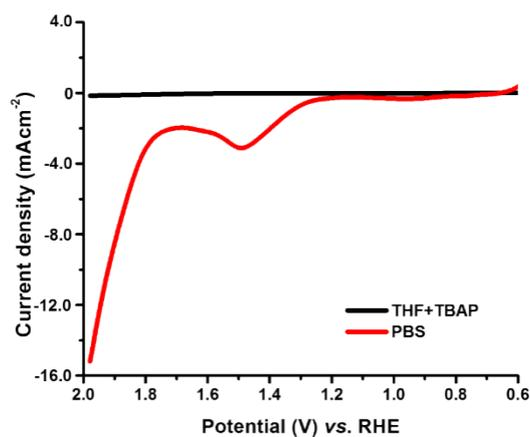
**Fig. S8** Overlaid LSV taken in aqueous (red curve) and non-aqueous solvent (black curve) at [Mn(OAc)(L)(cbpy)]-Au electrode.
