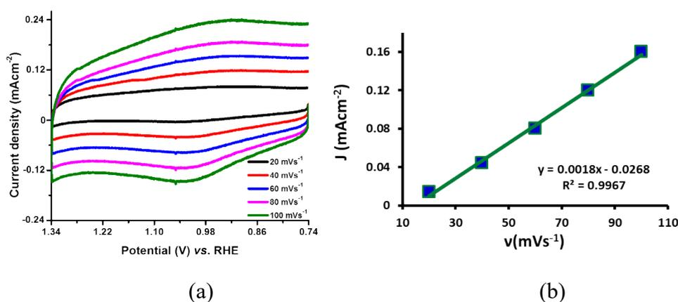
**Fig. S7** CVs of [Mn(OAc)(L)(cbpy)]-Au electrode in 0.1 M PBS at pH 7.0 at different scan rate (20-100 mVs<sup>-1</sup>) (a), A plot of current density *versus* scan rate (b).
