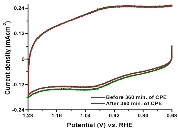
**Fig. S18** Overlaid CVs before and after CPE using [Mn<sup>III</sup>(OAc)(L)(cbpy)]-Au electrode (scan rate 100 mVs<sup>-1</sup>)
