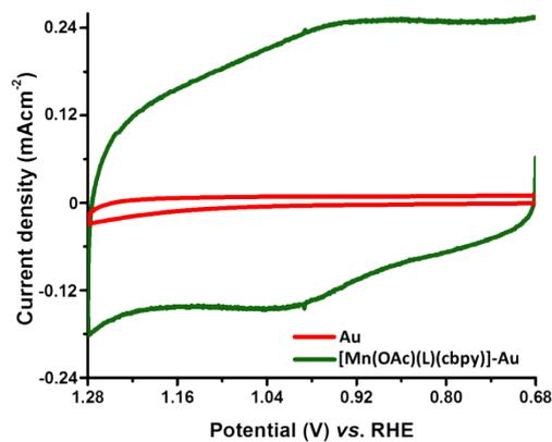
**Fig. S6** Overlaid CVs obtained at bare Au and [Mn(OAc)(L)(cbpy)]-Au electrodes in 0.1 M PBS at pH 7.0 (scan rate 1000 mVs<sup>-1</sup>).
