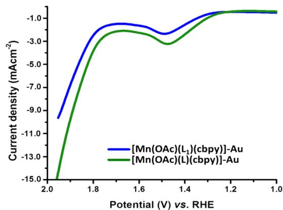
**Fig. S11** Overlaid LSV in 0.1 M PBS using  $[\text{Mn}(\text{OAc})(\text{L})(\text{cbpy})]\text{-Au}$  and  $[\text{Mn}(\text{OAc})(\text{L}_1)(\text{cbpy})]\text{-Au}$  electrode.
