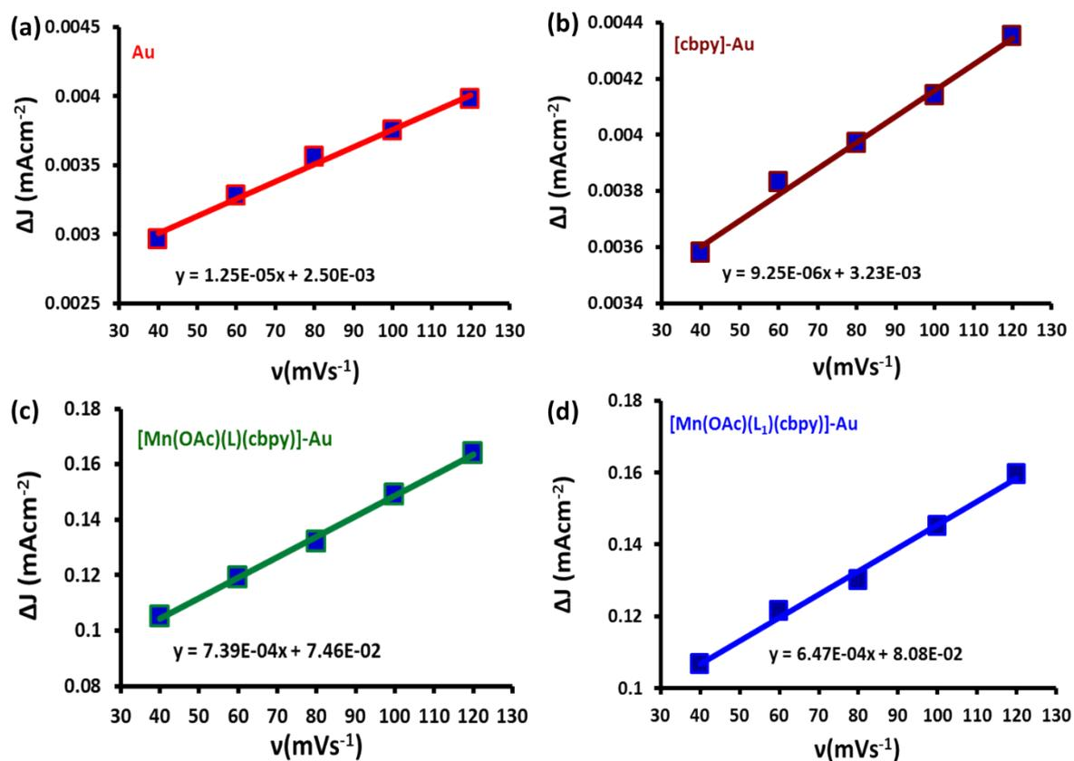
**Fig. 12** Plot of  $\Delta J$  ( $J_a - J_c$ ) versus scan rate ( $v$ ) for bare Au (a), cbpy-Au (b),  $[\text{Mn}(\text{OAc})(\text{L})(\text{cbpy})]\text{-Au}$  (c) and  $[\text{Mn}(\text{OAc})(\text{L}_1)(\text{cbpy})]\text{-Au}$  electrode. The slope ( $2C_{dl}$ ) were used to represent ECSA.
