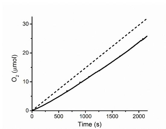
**Fig. S10** Oxygen evolution during the controlled potential electrolysis of water in a gas tight electrochemical cell under N<sub>2</sub> atmosphere (0.1 M PBS, pH 7.0) with [Mn(OAc)(L)(cbpy)]-Au electrode at an applied potential of + 1.48 V *versus* RHE. Dotted line denotes the theoretical oxygen evolution with 100 % efficiency.
