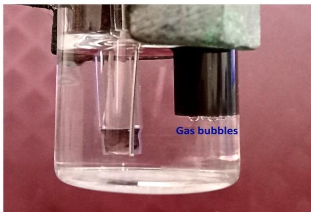
**Fig. S9** Formation of O<sub>2</sub> gas bubbles on the [Mn(OAc)(L)(cbpy)]-Au electrode after 25 repetitive runs.
