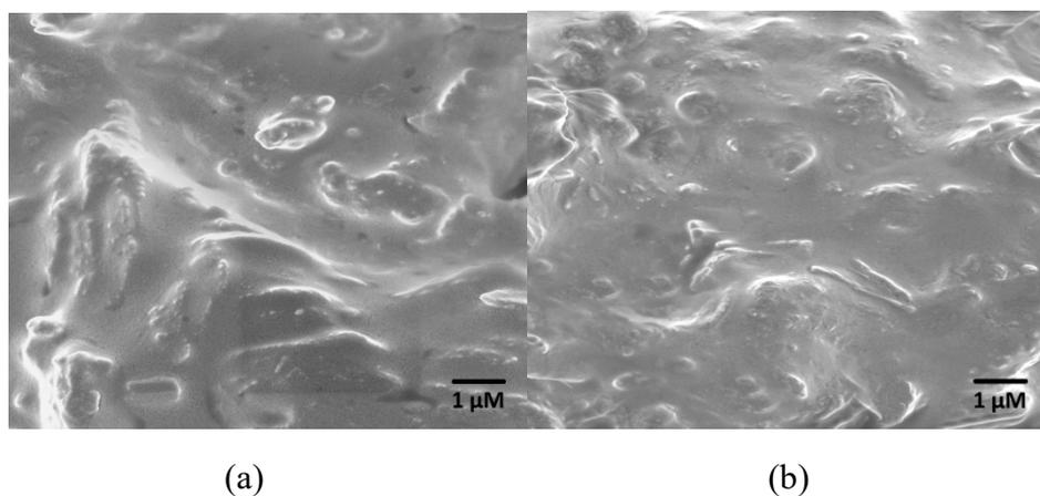
**Fig. 19** FE-SEM of [Mn<sup>III</sup>(OAc)(L)(cbpy)]-Au electrode before (a) and after (b) after six hours of CPE
