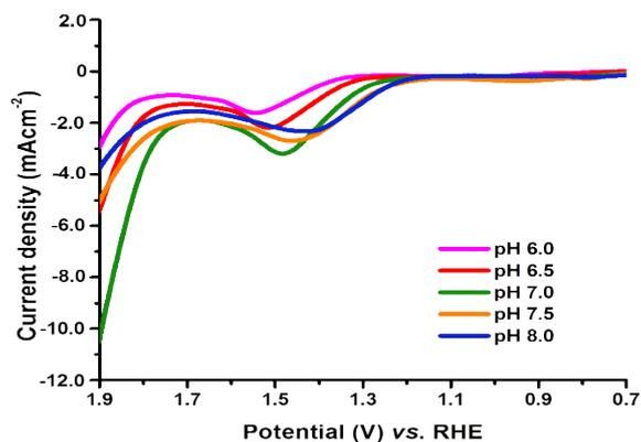
**Fig. S13** Overlaid LSV obtained at [Mn(OAc)(L)(cbpy)]-Au electrode with increasing pH from 6.0 to 8.0.
