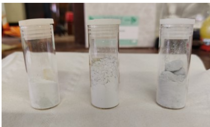
Figure S6. Sulfanilic acid obtained in experiments 10, 11 and 13 (from left to right) after dilution with water and filtration of the precipitated SA as the insoluble zwitterion.
