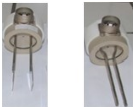
Figure S15. Rectangular (left) and cylindrical (right) stainless steel 316 electrodes.
