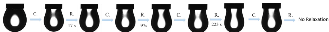
Figure S9. Snapshots of droplet's morphology evolution in an extraction- reinjection process, [Su-Py] = 0.01 M, [POSS-NH 2 ] = 1.0 g/L, pH=4.0. Scale bar: 2.0 mm.
