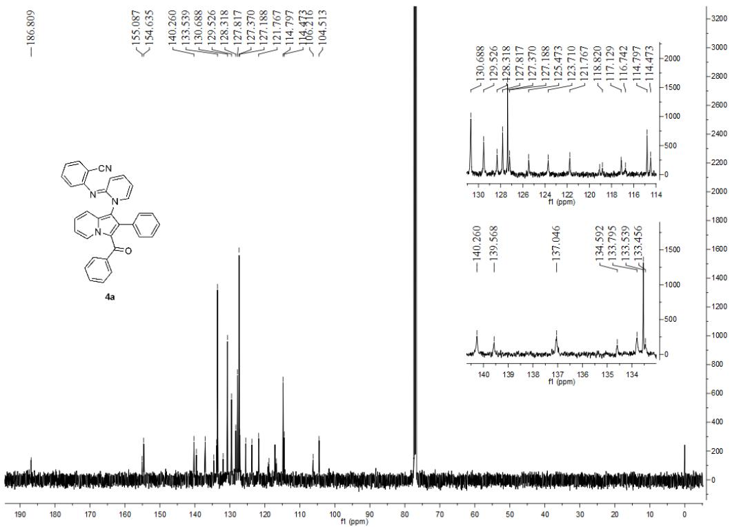
The  $^1\text{H}$  NMR ( $\text{CDCl}_3$ , 400 MHz) and  $^{13}\text{C}$  NMR ( $\text{CDCl}_3$ , 125 MHz) spectra of **4a**
