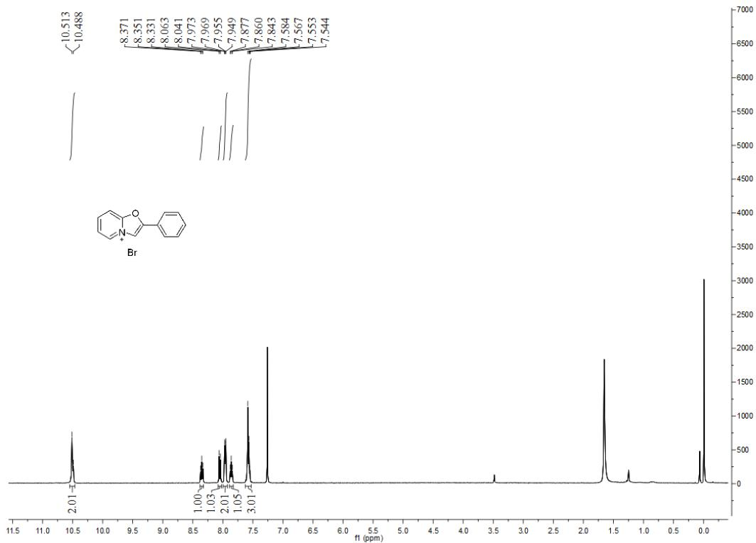
The  $^1\text{H}$  NMR ( $\text{CDCl}_3$ , 400 MHz) spectra of Intermediate B
