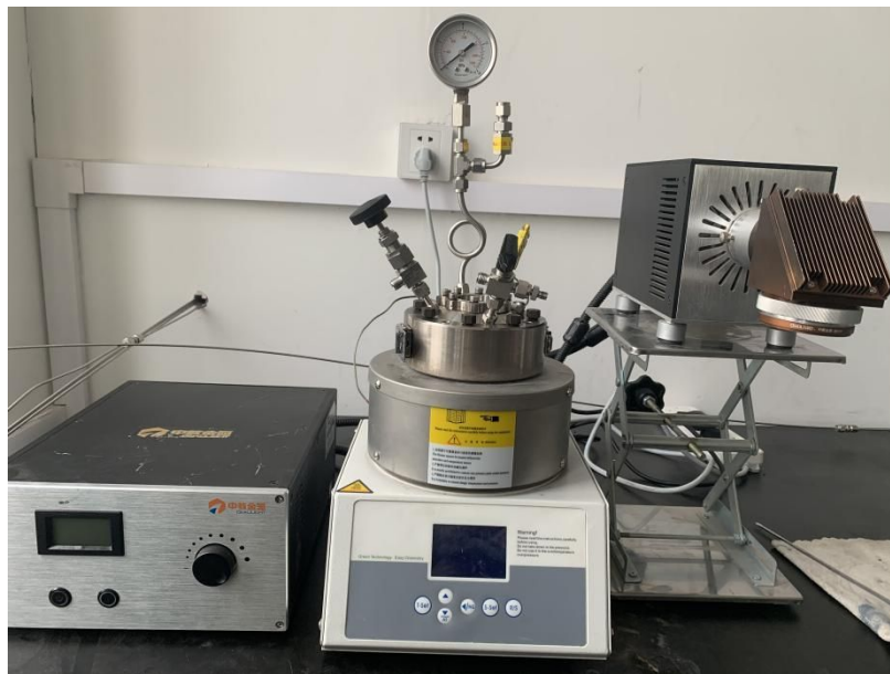
Fig. S1. Diagram of a photothermal synergistic catalytic reactor.
