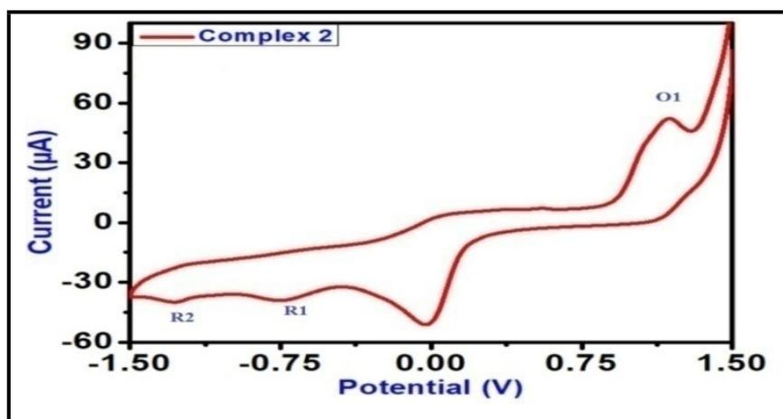
**Figure S17.** The cyclic voltammogram of complex **2** in dry acetonitrile at a  $100 \text{ mVs}^{-1}$  scan rate with Pt as the working electrode, Ag/AgCl as the reference electrode, and a  $0.1 \text{ (M)}$  solution of  $[\text{N}(\text{Bu})_4]\text{PF}_6$  as the supporting electrolyte.
