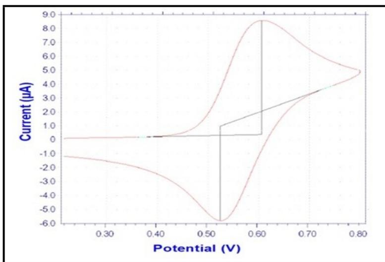
**Figure S18.** The cyclic voltammogram of **3** in dry acetonitrile at a  $100 \text{ mVs}^{-1}$  scan rate with Pt as the working electrode, Ag/AgCl as the reference electrode, and a 0.1(M) solution of  $[\text{N}(\text{Bu})_4]\text{PF}_6$  as the supporting electrolyte.
