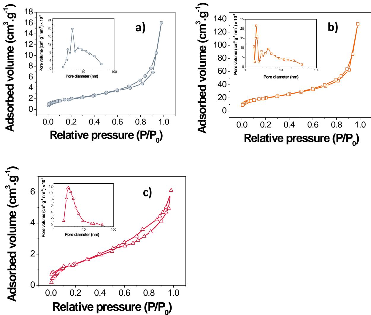
**Figure S2** – Type-IV sorption isotherms of samples: a) BM; b) BU, c) EM. In the inset is shown the pore-size distribution.
