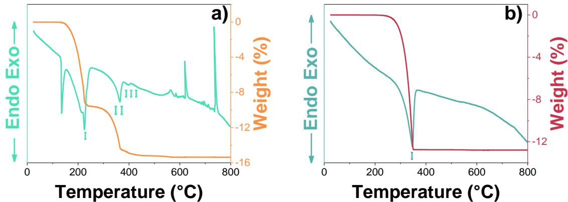
**Figure S1.** TG/DTA curves of urea and melamine pyrolysis in air (a, b respectively).
