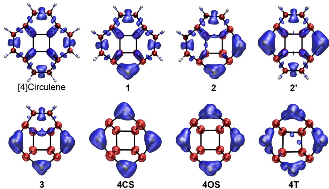
**Figure S19.** Calculated ICSS maps (isosurface value:  $\pm 28$  ppm) of [4]circulene and thia[4]circulenes **1–4**. Blue and red colored regions correspond to spaces with negative and positive NICS values, respectively.
