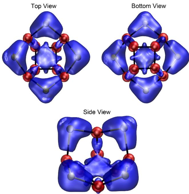
**Figure S18.** Calculated ICSS maps (isosurface value:  $\pm 19$  ppm) of **4T**. Blue and red colored regions correspond to spaces with negative and positive NICS values, respectively.
