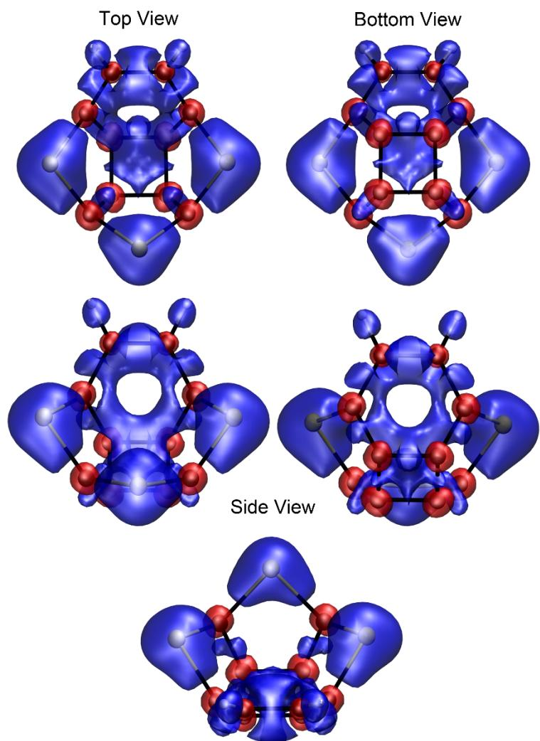
**Figure S15.** Calculated ICSS maps (isosurface value:  $\pm 19$  ppm) of **3**. Blue and red colored regions correspond to spaces with negative and positive NICS values, respectively.
