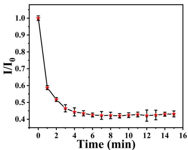
**Fig. S3** Fluorescence intensity ratio ( $I/I_0$ ) of Si-CDs at different incubating time from 0-15 min in the presence of  $Hg^{2+}$  (100  $\mu M$ ).
