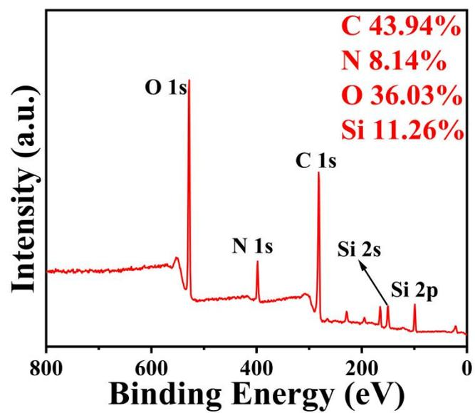
Fig. S1 Full survey XPS spectra of the Si-CDs.
