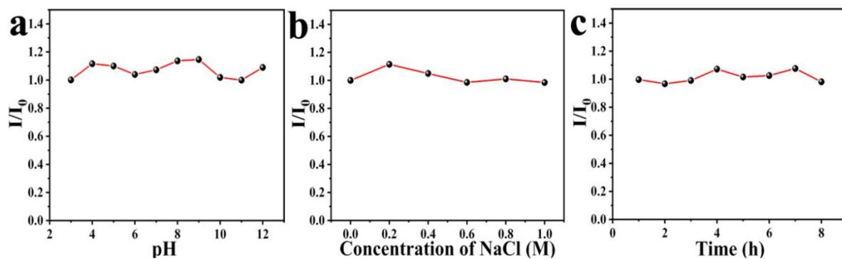
**Fig. S2** Fluorescence intensity ratio  $I/I_0$  of the Si-CDs under (a) different pH, (b) different salinity conditions, (c) different storage times.
