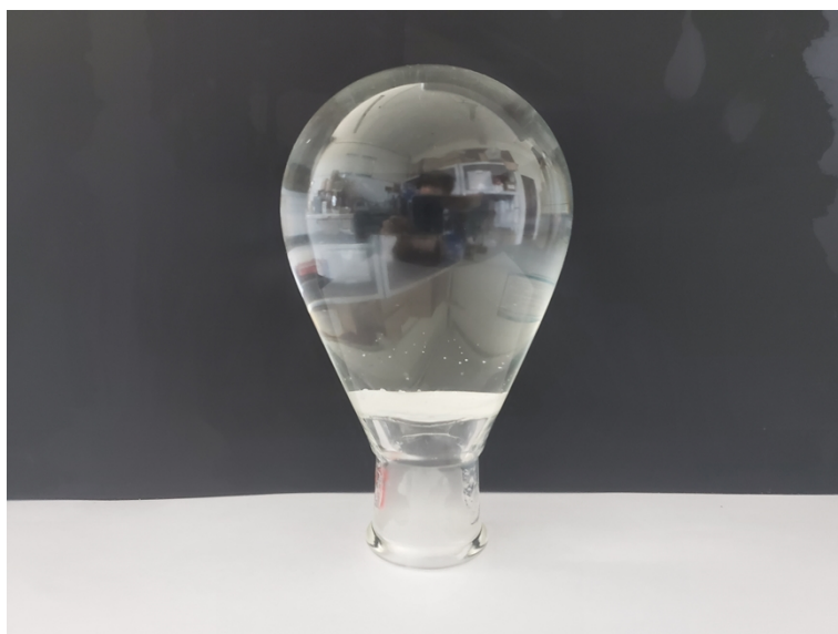
Figure S5. Mineral oil oleogel (2g, 2 wt%) of compound 1 holding the weight of 120 g of water in an inverted round-bottomed flask
