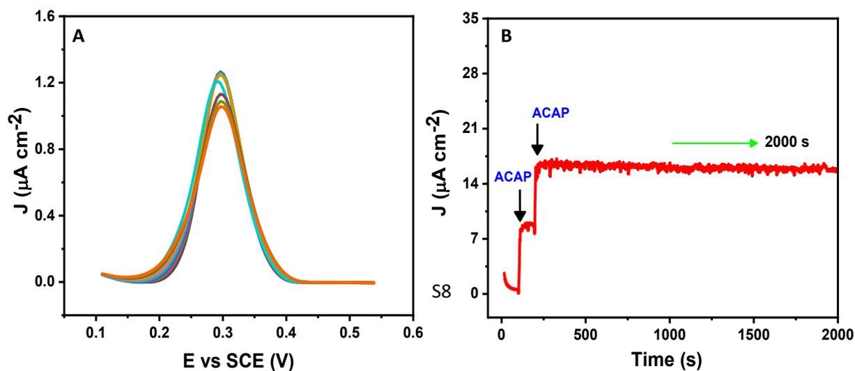
**Figure S10:** DPV interference effect of NP-MC with 10-fold NaCl, KCl, CaCl<sub>2</sub>, MgCl<sub>2</sub>, CuSO<sub>4</sub>, glucose and biomolecules with 5- fold excess of uric acid (UA), dopamine (DA) and ascorbic acid (AA) and (B) Dynamic amperometric stability response of NP-MC upto 2000 s.
