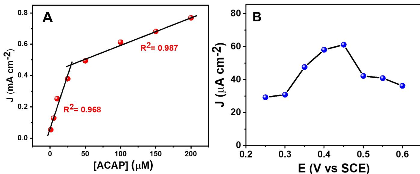
**Figure S9:** (A) linear calibration fit with different ACAP concentration in DPV (B) CA potential optimization study using an addition of 0.1 mM ACAP in 0.1 M PBS (pH-7.5) at various applied potential from 0.25 to 0.6 V over NP-MC/GCE.
