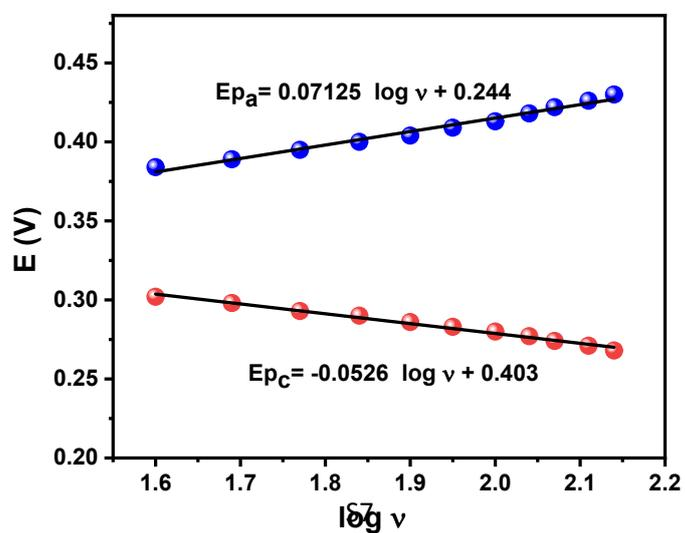
**Figure S8:** plot of  $E$  vs  $\log(v)$  of NP-MC in 0.1 mM ACAP at different scan rates from 5 to 140  $\text{mV s}^{-1}$ .
