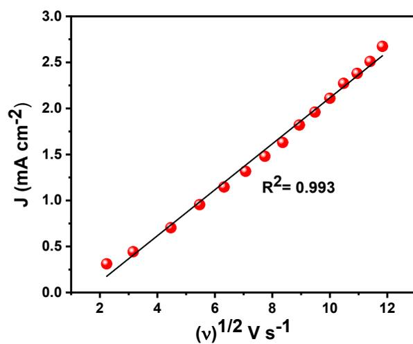
**Figure S7:** Plot of  $(J_{pa})$  vs  $(\nu)^{1/2}$  of NP-MC in 0.1 mM ACAP at different scan rates (5 to 140 mV s<sup>-1</sup>).
