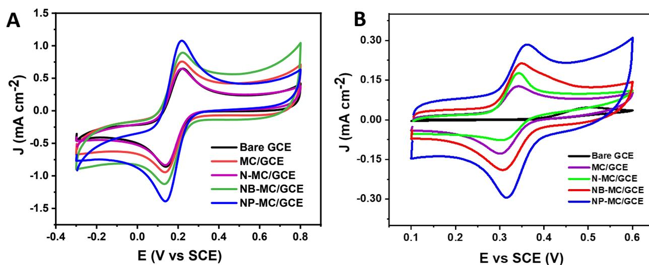
**Figure S5:** Cyclic voltammograms of modified electrodes at 25 mV s<sup>-1</sup>; (A) [Fe(CN)<sub>6</sub>]<sup>3-/4-</sup> redox system; (B) N<sub>2</sub>-saturated 0.1 M PBS with 0.2 mM ACAP.
