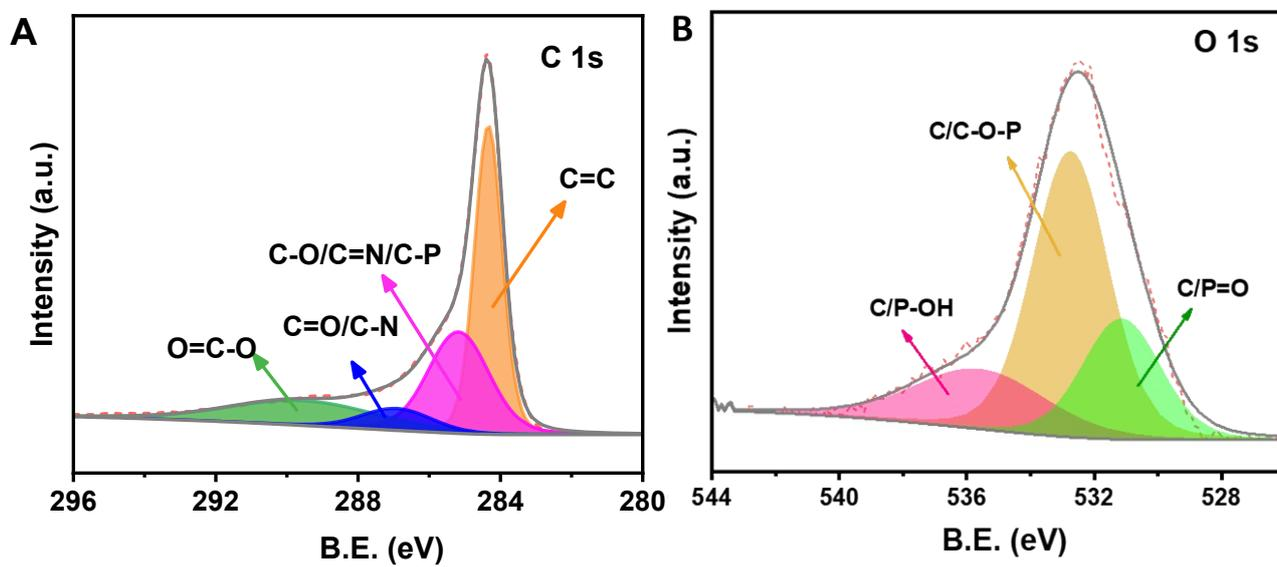
Figure S2: XPS spectra of C 1s (A) and O 1s (B) for NP-MC.
