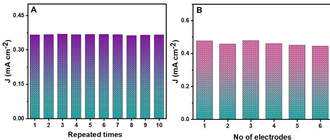
**Figure S11:** (A) Repeatability of NP-MC modified electrode for 10 times with a time interval of 3 min and (B) reproducibility of NP-MC modified electrode with 6 different electrodes in 0.1 mM ACAP.
