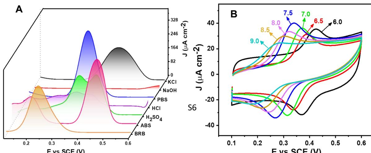
**Figure S6:** Cyclic voltammetric curves of NP-MC/GCE, (A) In different Supporting eletrolytes; (B) In different pH from 6.0-9.0.
