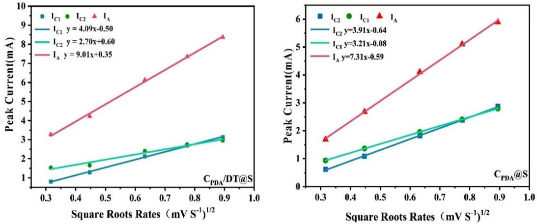
**Fig. S4** CV curves peak current of  $I_{C2}$  (cathodic reduction process,  $S_8 \rightarrow Li_2S_x$ ,  $3 \leq x \leq 8$ ),  $I_{C1}$  (cathodic reduction process,  $Li_2S_x \rightarrow Li_2S_2/Li_2S$ ) for three cathodes with multiple effects and  $I_A$  (anodic oxidation
