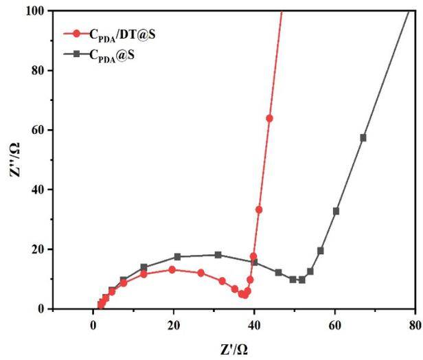
Fig. S3 EIS diagram after fitting of C<sub>PDA</sub>/DT and C<sub>PDA</sub>.
