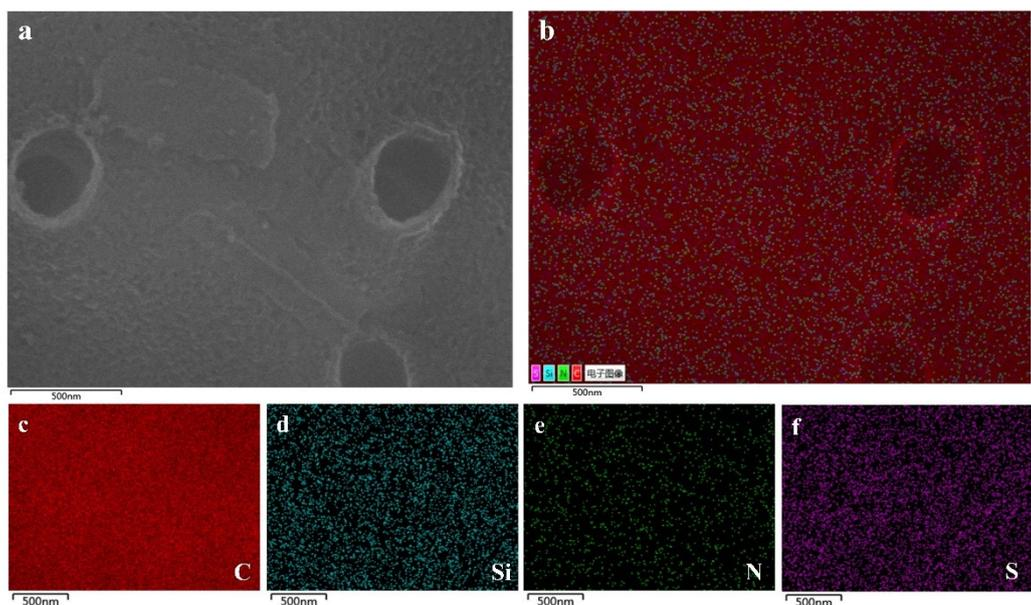
**Fig S5** (a) SEM images of CPAD/DT@S, and Elemental mapping images of (b) CPAD/DT@S for elements (c) C, (d) Si, (e) N, and (f) S respectively
