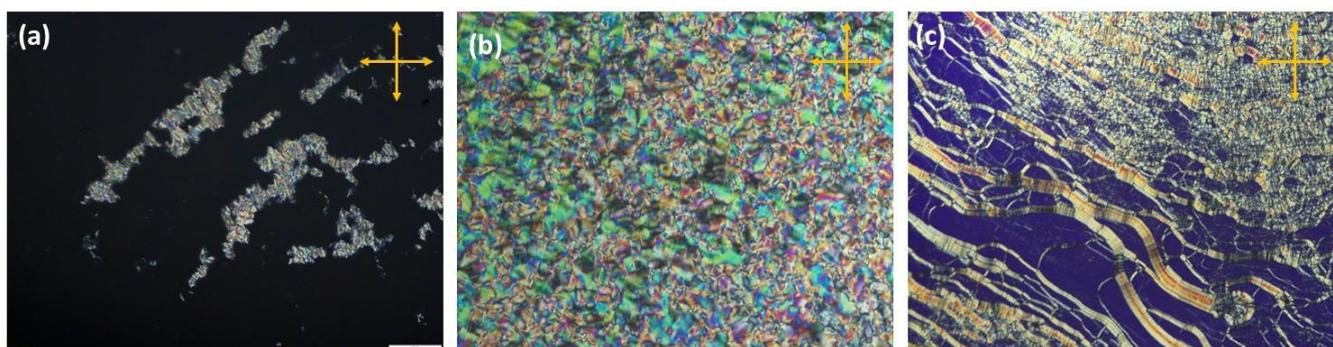
**Fig. S5:** POM micrographs of compound **5e** showing (a) SmA phase at 114 °C on heating, (b) TGB<sub>A</sub> phase at 117 °C on heating, (c) Cholesteric phase at 129 °C on heating.
