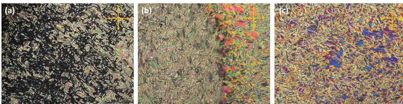
**Fig. S3:** POM micrographs of compound **5c** showing (a) smectic A phase at 77 °C on cooling, (b) Transition from TGB<sub>A</sub> to smectic A phase at 132.5 °C on cooling, (c) Cholesteric phase at 176 °C on cooling.
