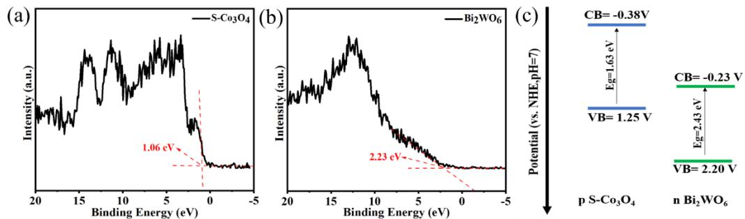
**Fig. S7** The maximum energy edge of the VB for (a) S-Co<sub>3</sub>O<sub>4</sub> and (b) Bi<sub>2</sub>WO<sub>6</sub>; and (c) a schematic illustration of the band structures of S-Co<sub>3</sub>O<sub>4</sub> and Bi<sub>2</sub>WO<sub>6</sub>.
