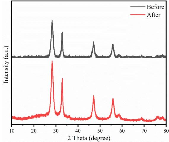
**Fig. S5** XRD patterns of SCB1 material before and after the recycle experiment.
