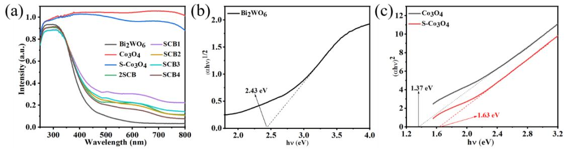
**Fig. S4** (a) UV-Vis DRS absorption spectra; (b) plots of  $(ahv)^{1/2}$  versus  $h\nu$  for pure  $\text{Bi}_2\text{WO}_6$ ; and (c) plots of  $(ahv)^2$  versus  $h\nu$  for pure  $\text{Co}_3\text{O}_4$  and S- $\text{Co}_3\text{O}_4$ .
