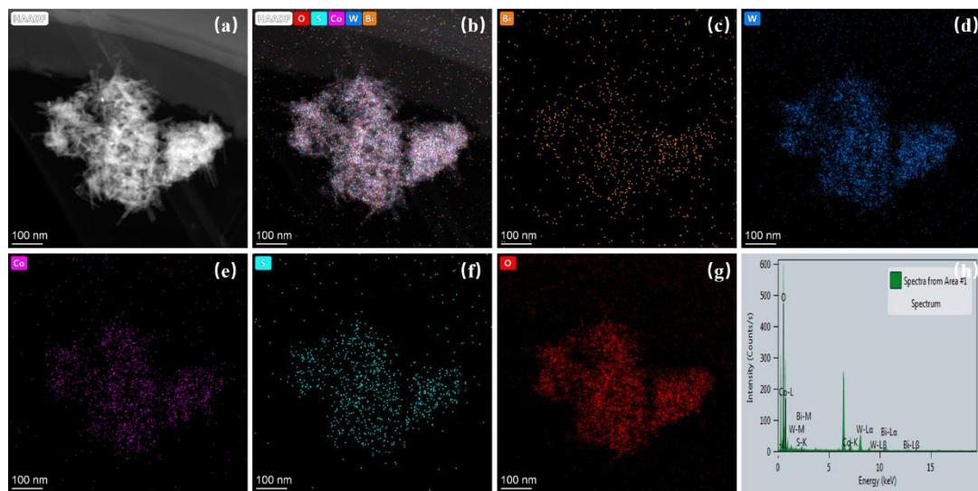
**Fig. S3** (a–h) EDS mapping images of S- $\text{Co}_3\text{O}_4/\text{Bi}_2\text{WO}_6$ .
