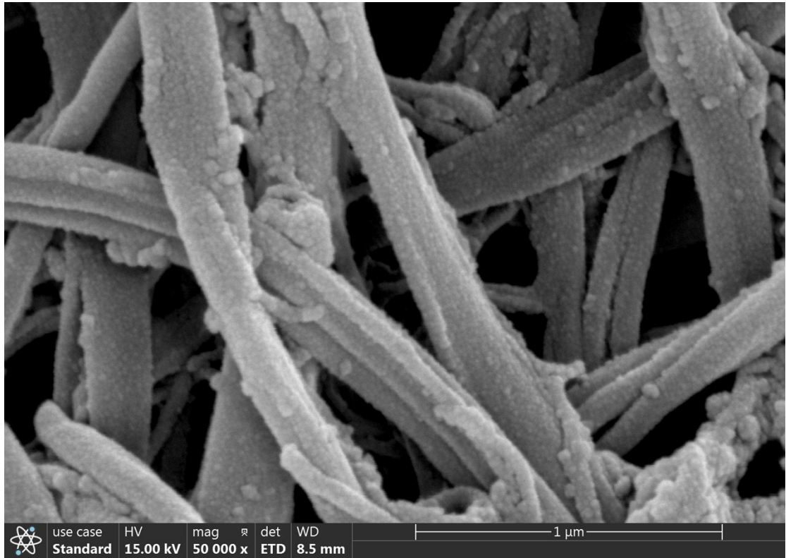
Figure S3. The SEM image of SNFs@PDA with SNFs mass ratio PDA is 1 to 1.5.
