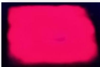
**Fig. S19** Photograph of CN1 coated glass slide taken under UV light ( $\lambda_{\text{ex}} = 365 \text{ nm}$ ).
