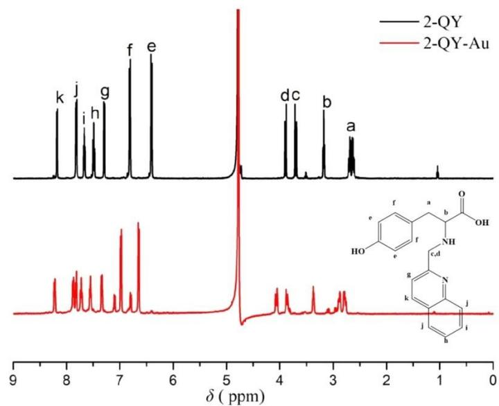
**Fig. S7**  $^1\text{H}$  NMR spectra of 2-QY and 2-QY-Au in  $\text{D}_2\text{O}$ .
