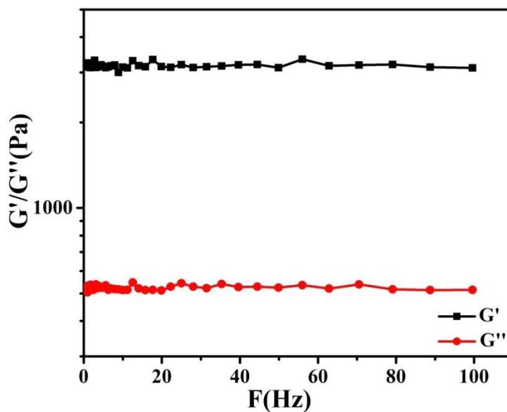
**Fig. S5** The dynamic frequency scan of 2-QY-Au NPs metallohydrogel.
