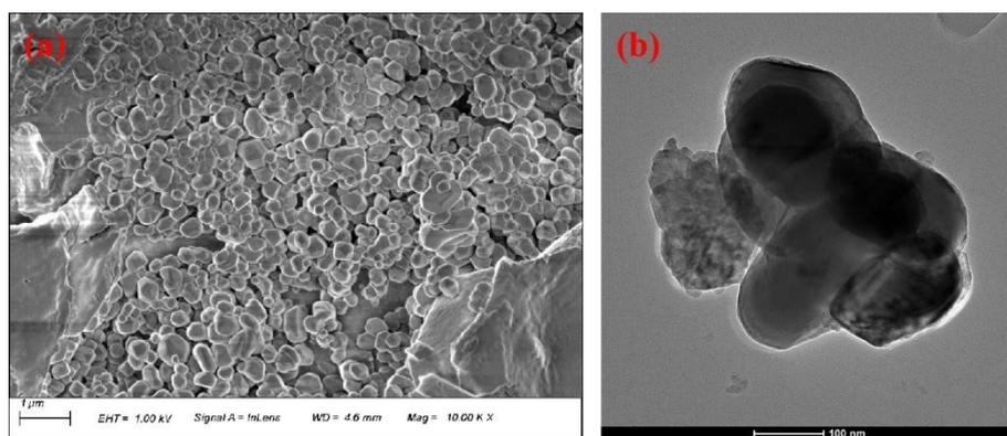
**Fig. S21** SEM and TEM images of Au NPs prepared from  $\text{NaBH}_4$  and  $\text{HAuCl}_4$ .
