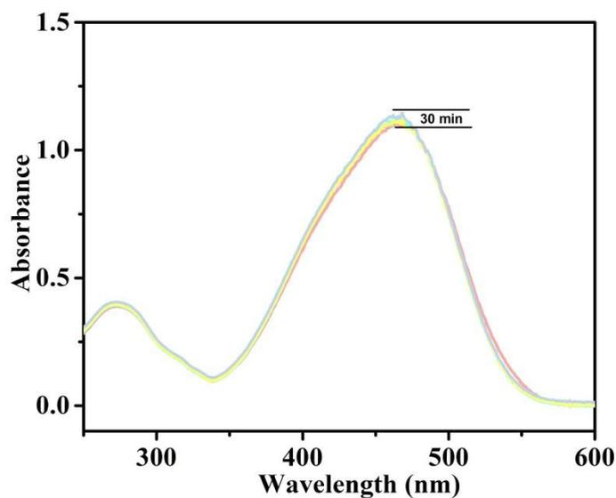
**Fig. S24** Time-dependent UV-vis spectra of MO reduced by NaBH<sub>4</sub> without 2-QY-Au NPs metallohydrogel.
