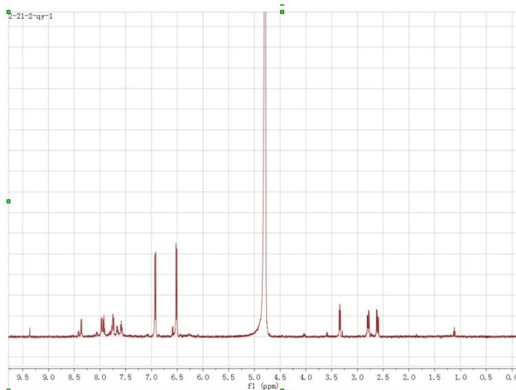
**Fig. S2**  $^1\text{H}$  NMR spectrum of the Schiff's base (precursor of 2-QY) in  $\text{D}_2\text{O}$ .
