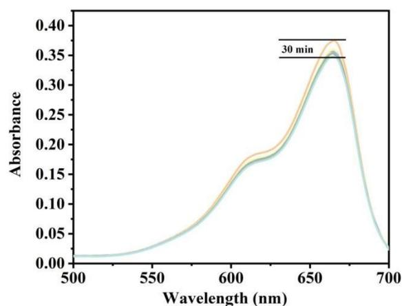
**Fig. S19** Time-dependent UV-vis spectra of MB reduced by 2-QY without  $\text{NaBH}_4$  and Au NPs. Reaction conditions: MB ( $10 \mu\text{M}$ ), Au NPs ( $0.02 \mu\text{M}$ ) and neutral pH.
