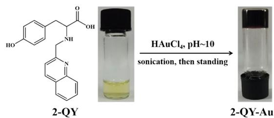
**Fig. S4** The structure of 2-QY and the formation of 2-QY-Au NPs metallohydrogel.
