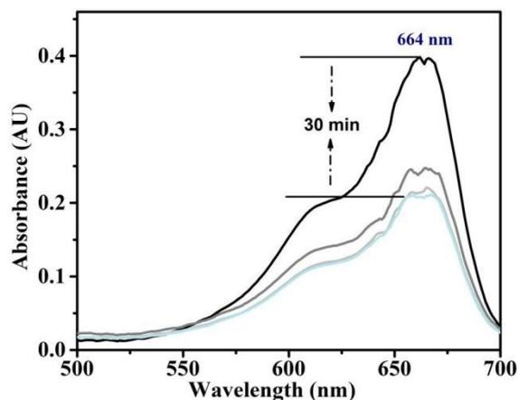
**Fig. S20** Time-dependent UV-vis spectra of MB reduced by  $\text{NaBH}_4$  in the presence of Au NPs prepared through  $\text{NaBH}_4$  reduction. Reaction concentration:  $\text{NaBH}_4$  ( $100 \mu\text{M}$ ), MB ( $10 \mu\text{M}$ ), Au NPs ( $0.02 \mu\text{M}$ ).
