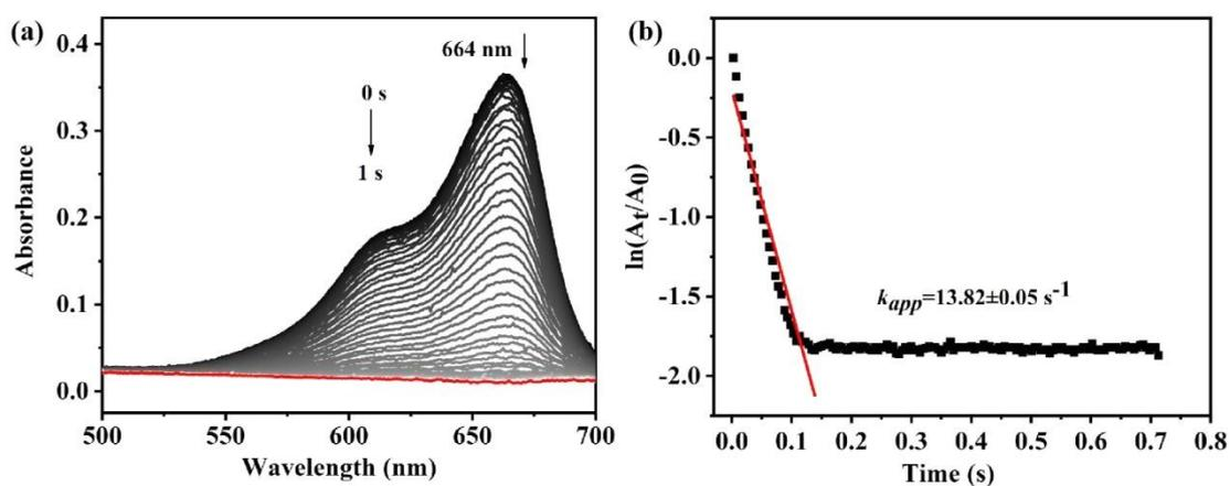
**Fig. S22** Time-dependent UV-vis spectra of MB reduced by  $\text{NaBH}_4$  (a) with 2-QY-Au NPs Xerogel, (b) the fitted curve of  $\ln(A_t/A_0)$  versus reaction time for the degradation of MB with 2-QY-Au NPs metallohydrogel. Reaction conditions: initial MB concentration = 0.01 mM,  $\text{NaBH}_4$  = 0.1 mM, catalyst dosage = 0.12 mg/mL, neutral pH, room temperature.
