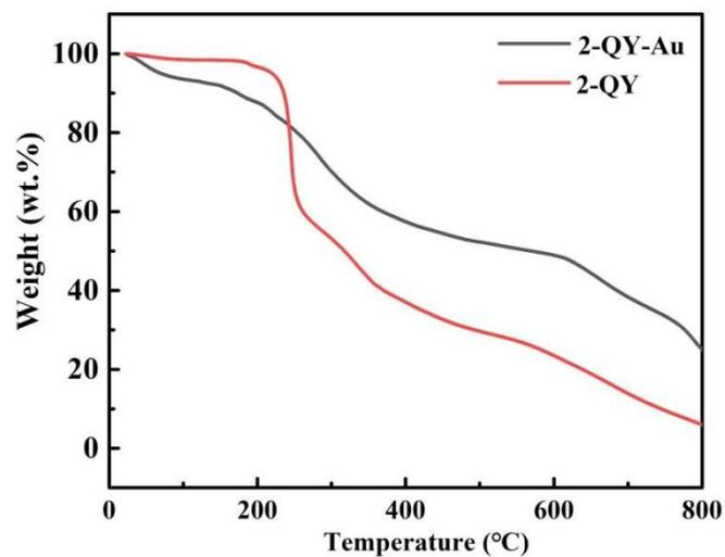
**Fig. S11** Thermogravimetric analysis (TGA) thermogram of 2-QY powder and 2-QY-Au NPs metallohydrogel.
