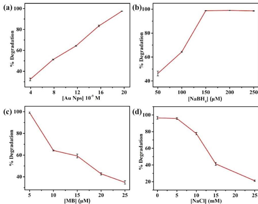
**Fig. S23** The percentage of degradation of MB within 0.2 s at different effect factors (a) catalyst dose, (b) NaBH<sub>4</sub> concentration, (c) initial dye concentration, and (d) ionic strength. Reaction conditions: effect of catalyst dosage, [MB] = 0.01 mM, [NaBH<sub>4</sub>] = 0.1 mM; effect of NaBH<sub>4</sub>: [MB] = 0.01 mM, [Au NPs] = 11.76 × 10<sup>-9</sup> M; effect of initial dye concentration and effect ionic strength: [MB] = 0.01 mM, [Au NPs] = 11.76 × 10<sup>-9</sup> M.
