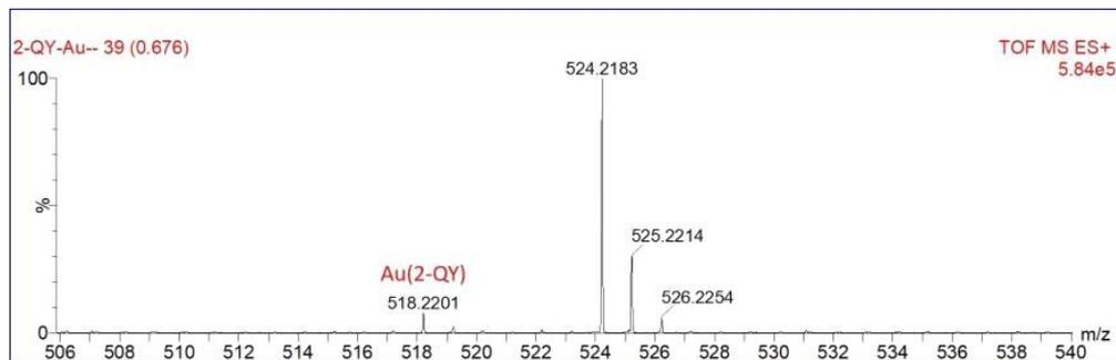
**Fig. S10** ESI-MS spectra of 2-QY-Au complex, Calculated: 517.3 Da; Observed: 518.2 Da ( $[\text{Au}(2\text{-QY}) + \text{H}]$ ).
