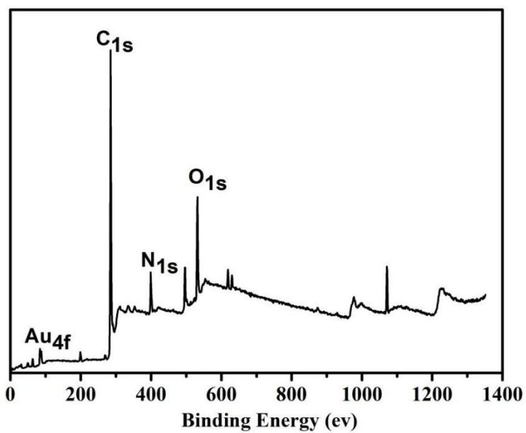
Fig. S17 X-Ray photoelectron spectroscopy of 2-QY-Au xerogel.
