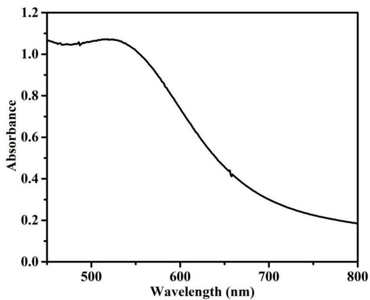
**Fig. S15** UV-vis spectrum of the diluted 2-QY-Au metallohydrogel.
