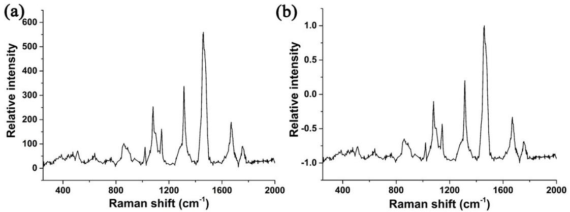
**Figure S11** (a) Raman spectrum after wavelet denoising (b) normalized spectrum of brand 1 (integration time: 80 s).
