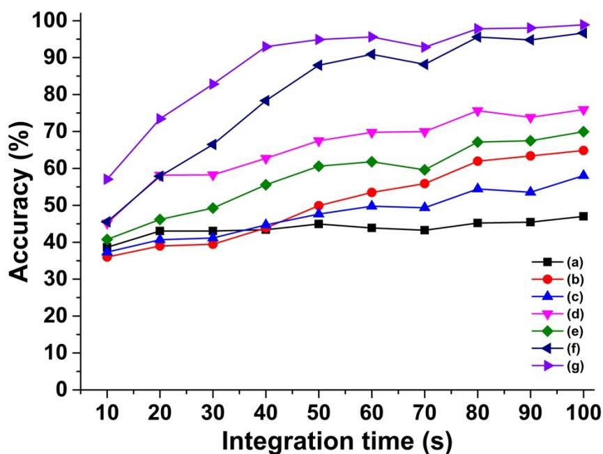
**Figure S13** The recognition results are based on (a) original spectrum, (b) wavelet denoising, (c) normalization (d) principal component analysis (e) wavelet denoising combined with normalization, (f) normalization combined with principal component analysis (g) wavelet denoising, normalization and principal component analysis. (the number of hidden layer neurons is 250).
