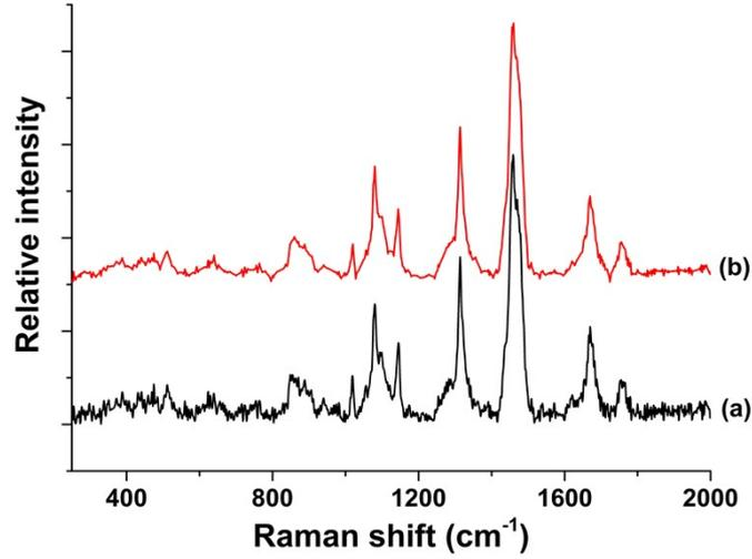
**Figure S10** (a) Original Raman spectrum (b) after wavelet denoising of brand 1 (integration time: 80 s).
