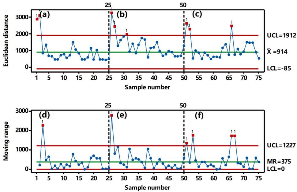
**Figure S8** Quality fluctuation individual value of brand 1 (a), brand 2 (b), and brand 3 (c) and moving range of brand 1 (d), brand 2 (e), and brand 3 (f) based on calculation results of Raman spectral Euclidean distance (integration time: 90 s), respectively. UCL=upper control limit; LCL=lower control limit;  $\overline{MR}$ =the average value of moving range control chart.  $\bar{x}$ =the average value of individual control chart.
