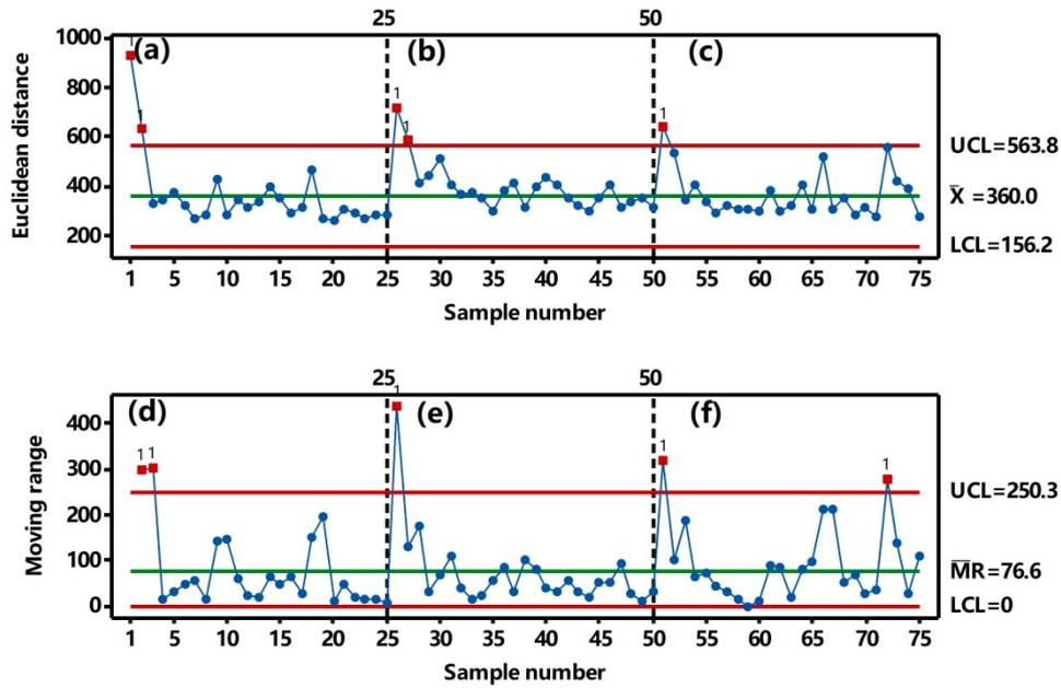
**Figure S2** Quality fluctuation individual value of brand 1 (a), brand 2 (b), and brand 3 (c) and moving range of brand 1 (d), brand 2 (e), and brand 3 (f) based on calculation results of Raman spectral Euclidean distance (integration time: 20 s), respectively. UCL=upper control limit; LCL=lower control limit;  $\bar{MR}$  =the average value of moving range control chart.  $\bar{X}$  =the average value of individual control chart.
