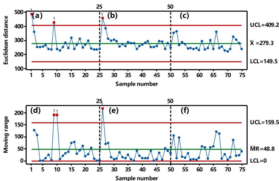
**Figure S1** Quality fluctuation individual value of brand 1 (a), brand 2 (b), and brand 3 (c) and moving range of brand 1 (d), brand 2 (e), and brand 3 (f) based on calculation results of Raman spectral Euclidean distance (integration time: 10 s), respectively. UCL=upper control limit; LCL=lower control limit;  $\overline{MR}$ =the average value of moving range control chart.  $\bar{x}$ =the average value of individual control chart.
