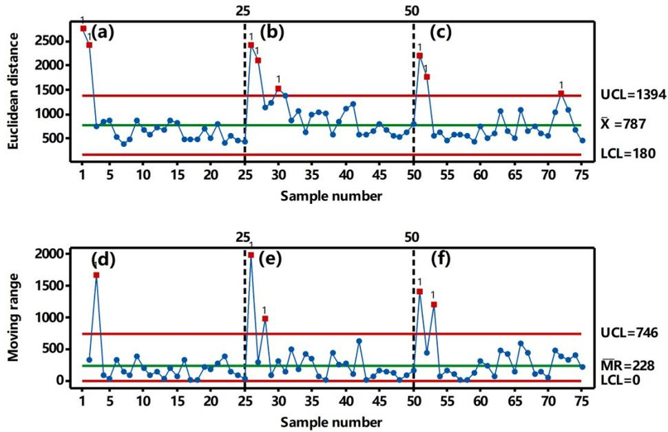
**Figure S7** Quality fluctuation individual value of brand 1 (a), brand 2 (b), and brand 3 (c) and moving range of brand 1 (d), brand 2 (e), and brand 3 (f) based on calculation results of Raman spectral Euclidean distance (integration time: 70 s), respectively. UCL=upper control limit; LCL=lower control limit;  $\overline{MR}$  =the average value of moving range control chart.  $\bar{x}$  =the average value of individual control chart.
