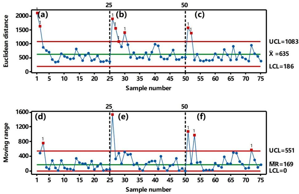
**Figure S5** Quality fluctuation individual value of brand 1 (a), brand 2 (b), and brand 3 (c) and moving range of brand 1 (d), brand 2 (e), and brand 3 (f) based on calculation results of Raman spectral Euclidean distance (integration time: 50 s), respectively. UCL=upper control limit; LCL=lower control limit;  $\overline{MR}$  =the average value of moving range control chart.  $\bar{x}$  =the average value of individual control chart.
