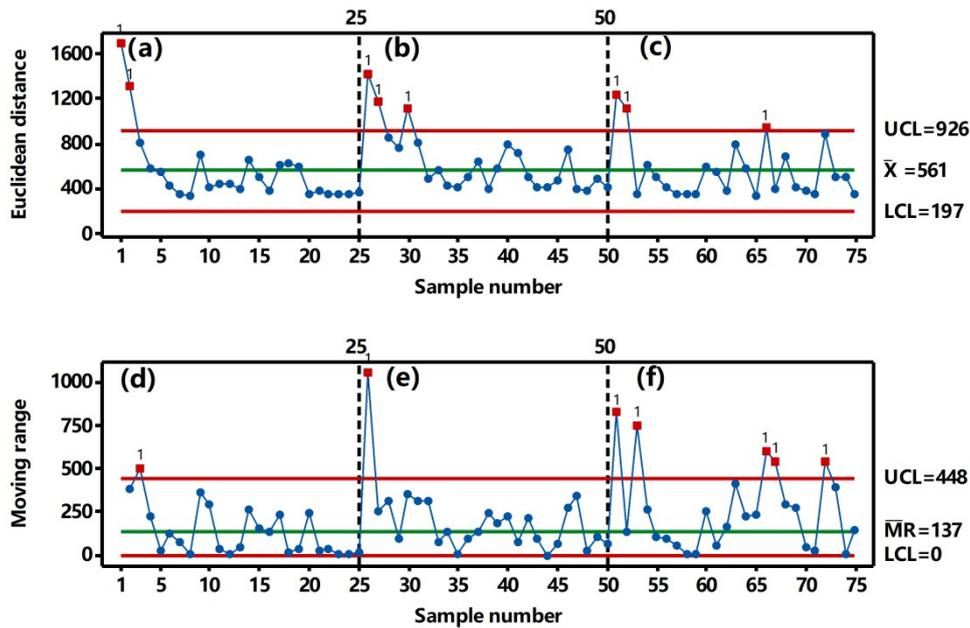
**Figure S4** Quality fluctuation individual value of brand 1 (a), brand 2 (b), and brand 3 (c) and moving range of brand 1 (d), brand 2 (e), and brand 3 (f) based on calculation results of Raman spectral Euclidean distance (integration time: 40 s), respectively.
