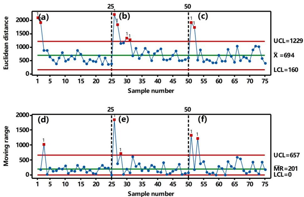
**Figure S6** Quality fluctuation individual value of brand 1 (a), brand 2 (b), and brand 3 (c) and moving range of brand 1 (d), brand 2 (e), and brand 3 (f) based on calculation
