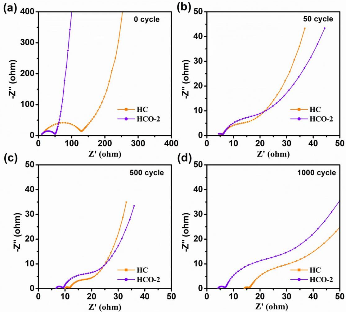
**Fig. S4.** EIS spectra of original HC and HCO-2 electrodes and after (a) 0, (b) 50, (c) 500, and 1000 cycles.
