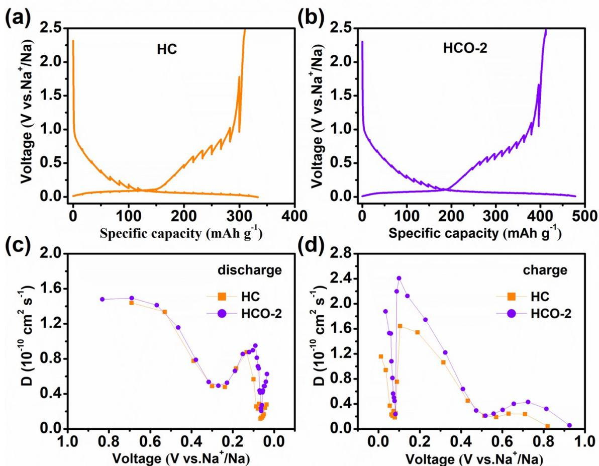
**Fig. S3.** The GITT curves of (a) HC and (b) HCO-2. The corresponding calculated Na<sup>+</sup> diffusion coefficients curves of (c) HC and (d) HCO-2.
