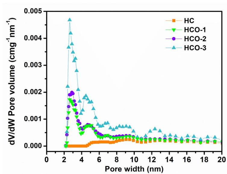
**Fig. S2.** NLDFT pore size distribution of HC, HCO-1, HCO-2 and HCO-3.
